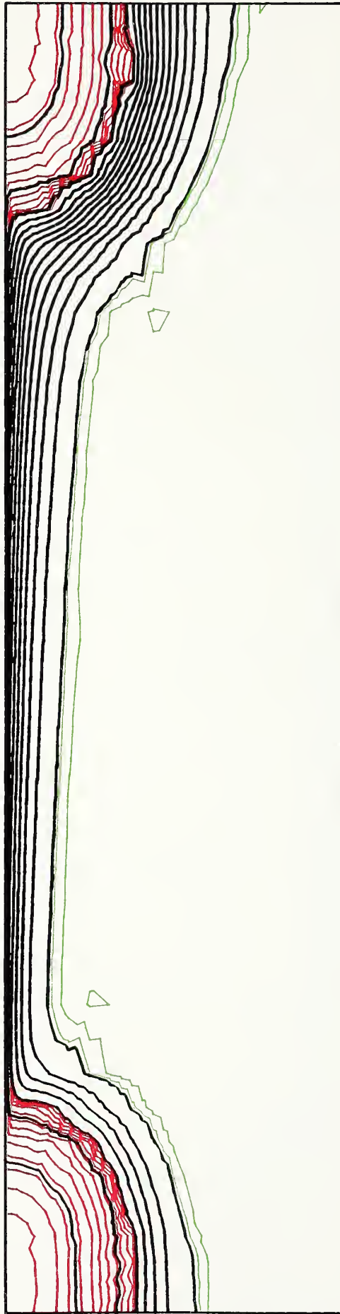
Figure 11. The potential, electron density, and hole density in the 8.17 - \mu\text{m} transistor at a bias of V_g = 2.0 V and V_d = 2.0 V.
