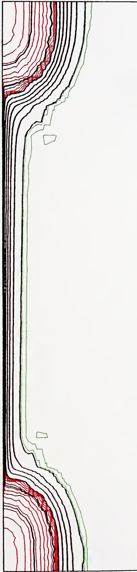
Figure 10. The potential, electron density, and hole density in the 8.17 - \mu\text{m} transistor at a bias of V_g = 2.0 V and V_d = 0.25 V.
