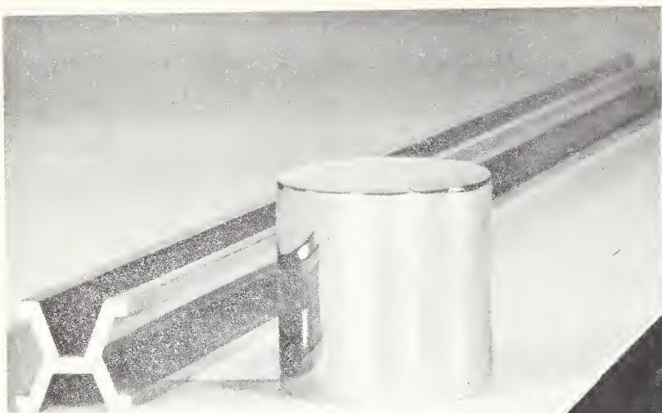
International metre and international kilogram of 1889 (life-size front views).
