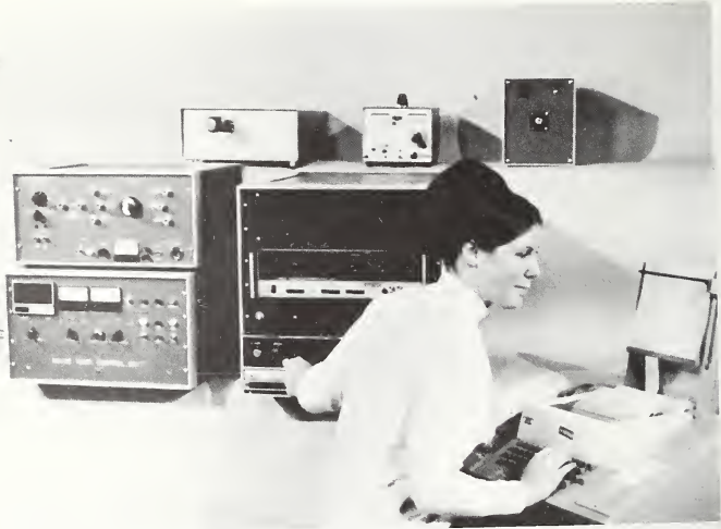
Figure 12. Automated Y-factor mm-wave noise measurement system.
