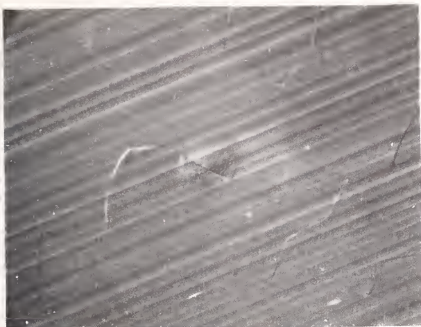
Figure 2. Nomarski micrographs of damage sites showing slip on a diamond-machined OFHC copper surface with the initial sample temperature at 133^{\circ}\text{K} in (a) and 300^{\circ}\text{K} in (b). No differences in morphology are evident.
