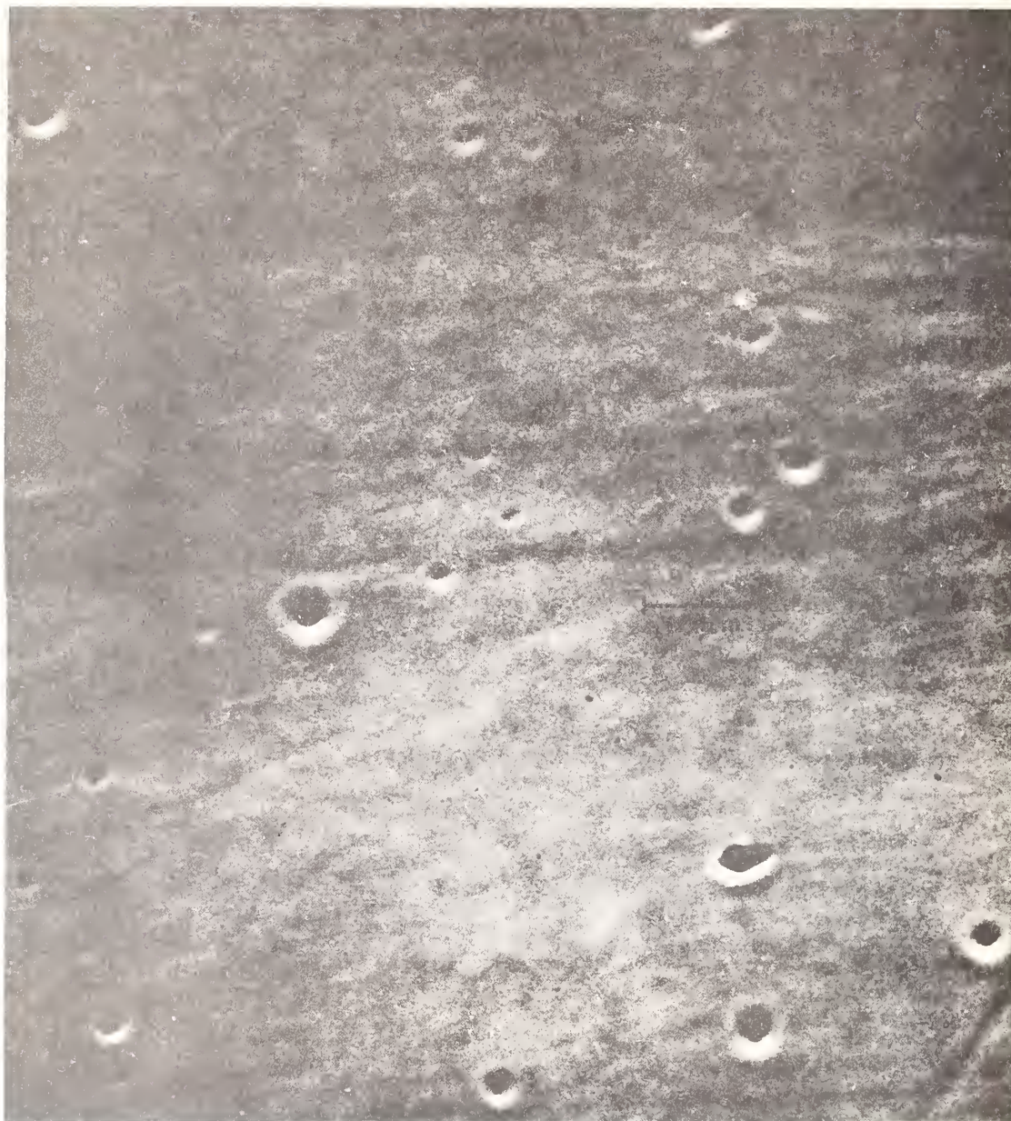
Figure 6. Onset of unipolar arc crater formation on highly polished stainless steel.
