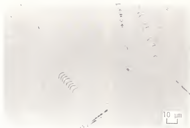
Figure 9. Nomarski micrograph of well-polished fused silica [1] after 5 minutes etching with 5 % HF.
