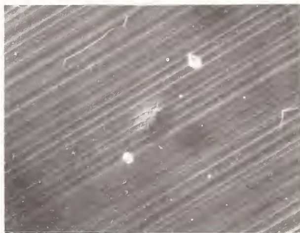
Figure 2. Nomarski micrographs of damage sites showing slip on a diamond-machined OFHC copper surface with the initial sample temperature at 133^{\circ}\text{K} in (a) and 300^{\circ}\text{K} in (b). No differences in morphology are evident.
