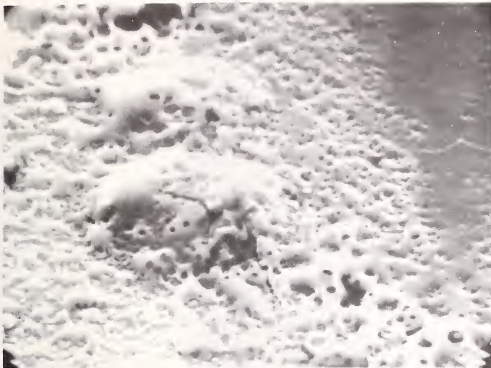
Figure 12. Unipolar arc craters on TiC coated SS304 after irradiation at 300 \text{ MW/cm}^2 .
