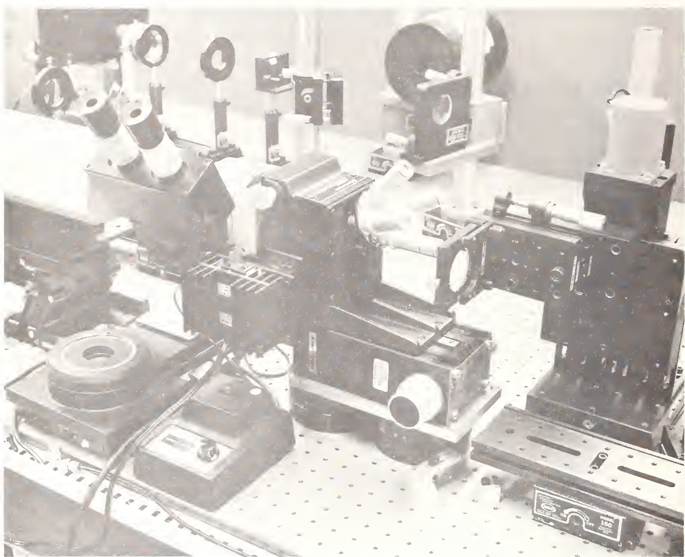
Figure 2. Photograph of test section. Sample holder on X-Y steppers is located a few cm from objective of microscope (center). Beam enters from right.
