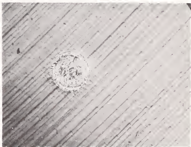
Figure 3. Nomarski micrographs of damage sites showing cratering on a diamond-machined electroplated gold surface with the initial sample temperature at 139^{\circ}\text{K} in (a) and 276^{\circ}\text{K} in (b). No differences in morphology are evident.
