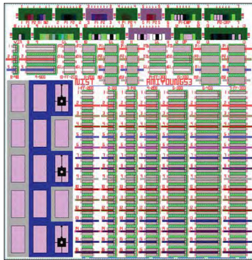
Figure 2. CMOS test chip design incorporating thickness test structures, cantilevers, fixed-fixed beams, and tensile test structures.
