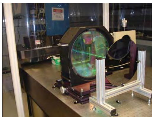
Figure 2. Test arm of the IR 3 interferometer: shown are the collimator lens and the beam expander together with a 300 mm silicon wafer. The insensitivity of the measurement to vibration permits the use of a simple wafer mount.
