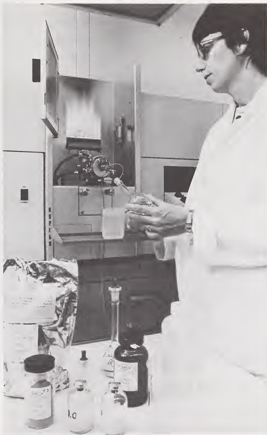
◀ These Butler aspirates a solution of an SRM into the flame atomic absorption (AA) spectrometer. Major and minor elements are determined in a variety of SRMs using flame AA, while trace elements are determined using electrothermal atomization AA.
