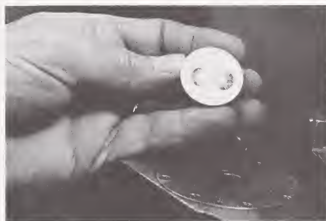
John Norris removes a ferrous SRM from the stand of a controlled waveform spark emission polychrometer. Analytical results for multiple burn spots are used to assess SRM homogeneity.
