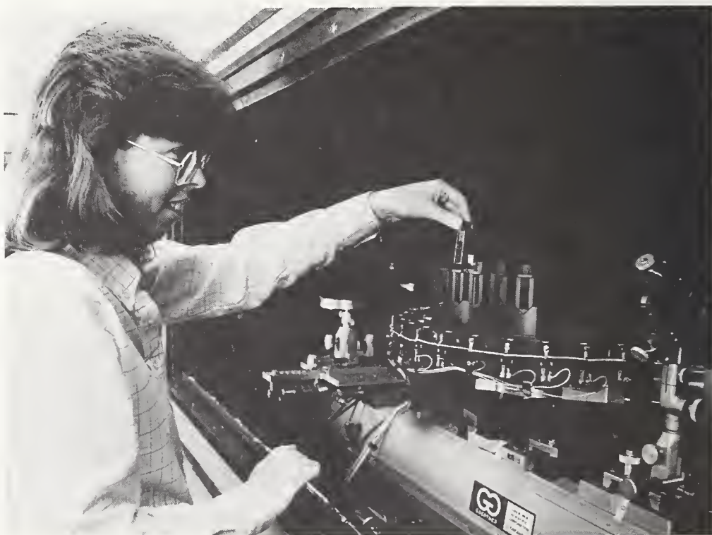
Melody Smith calibrates SRM 930D, Glass Filters for Spectrophotometry. This SRM is a reference source for the verification of the transmittance and absorbance scales of spectrophotometers.
