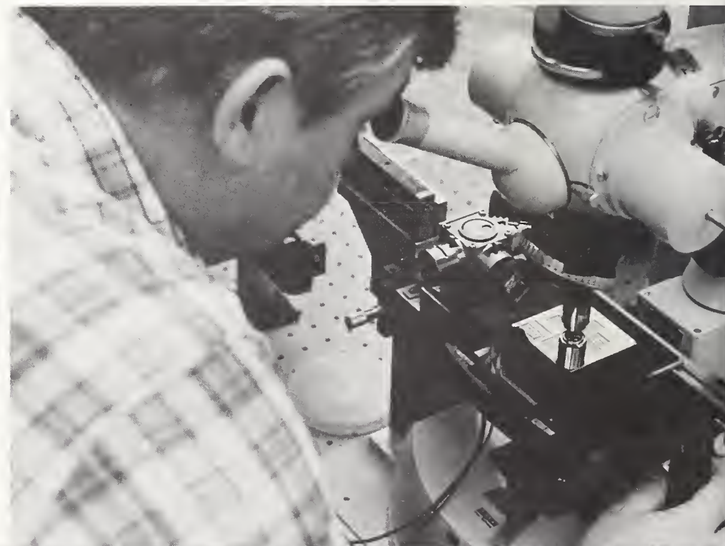
Samuel Jones examines SRM 475, Optical Microscope Linewidth Measurement Standard, used in calibrating optical microscopes that measure linewidths from 0.5 to 10 \mu\text{m} .
