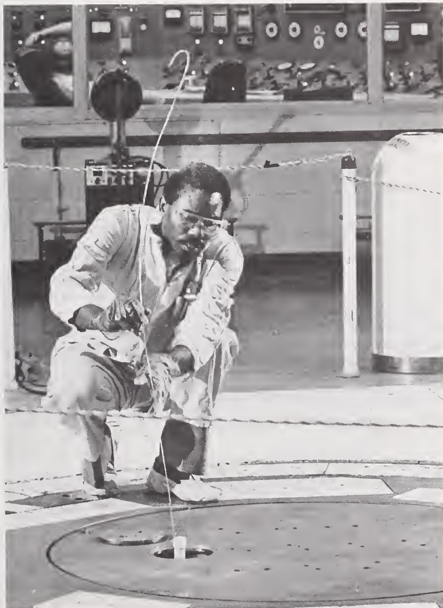
NBS uses its research reactor for a variety of research work, including the analysis of environmental and biological SRM's. Thomas Gills inserts a sample into the reactor.
