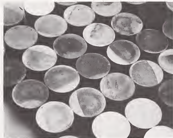
▲ After rough castings are separated from the original grid, individual disks of SRM C1146a, White Cast Iron, are polished for use in optical emission and x-ray spectrometric analysis.
