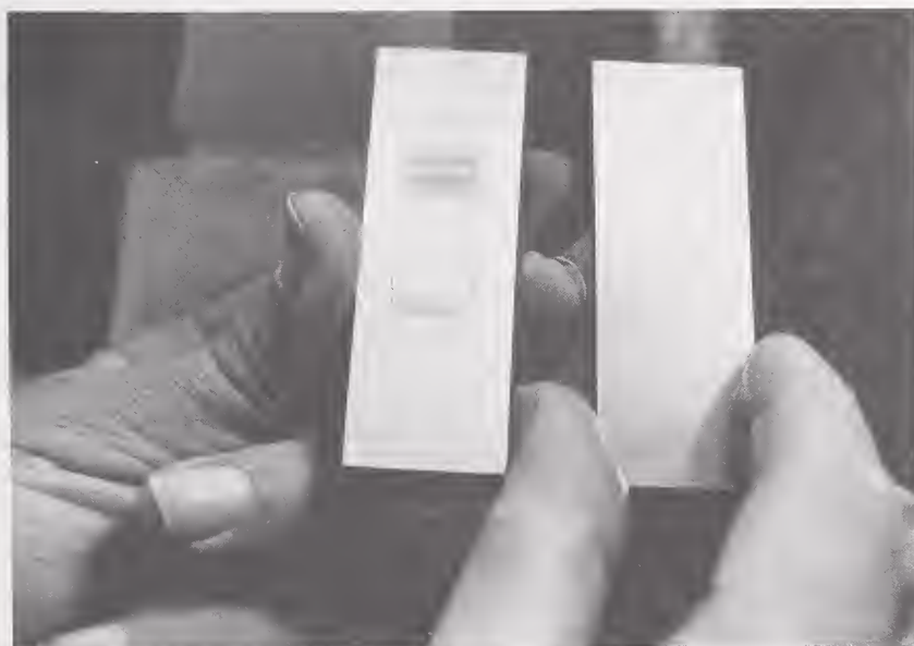
Tool Steel Abrasive Wear Standard, SRM 1857, is intended for use with the dry sand/rubber wheel abrasion wear method as described in ASTM Standard Practice G65-81, Procedure A.
