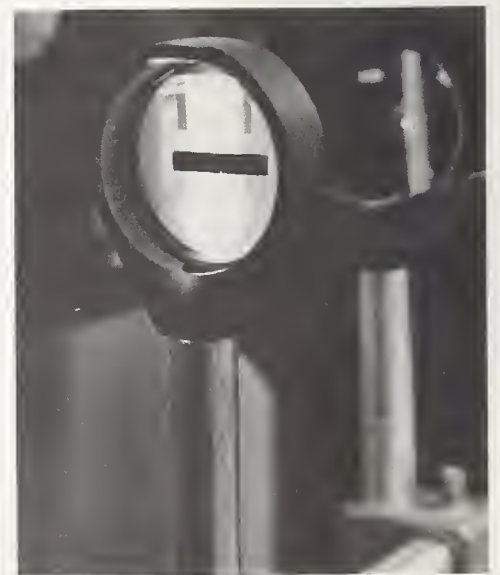
Robert Watters checks the alignment of the plasma flame image on the entrance mask of the inductively coupled plasma (ICP) spectrometer. A five-millimeter aperture is centered at the observation height of the plasma. This height is chosen to assure the best sensitivity for simultaneous multielement analysis using the ICP.
