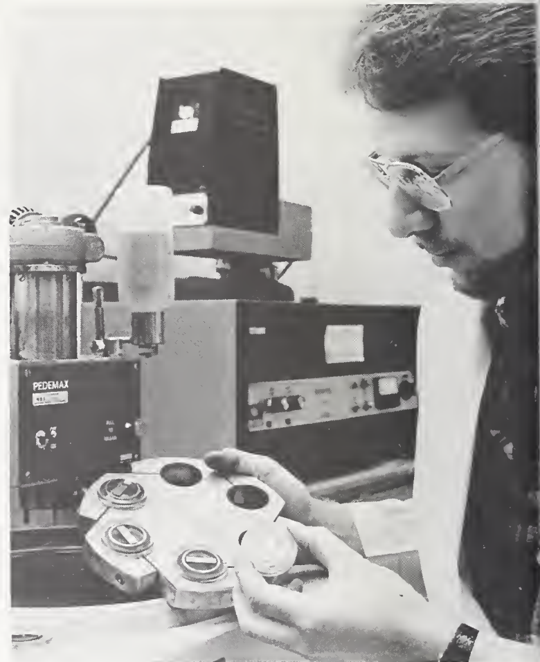
The standard being examined by David Kelley is SRM 1850, Penetrant Test Block. The sensitivity and performance of liquid dye penetrants and dye penetrant crack detection systems, as well as other systems and devices for surface defect detection may be checked by using this SRM.
