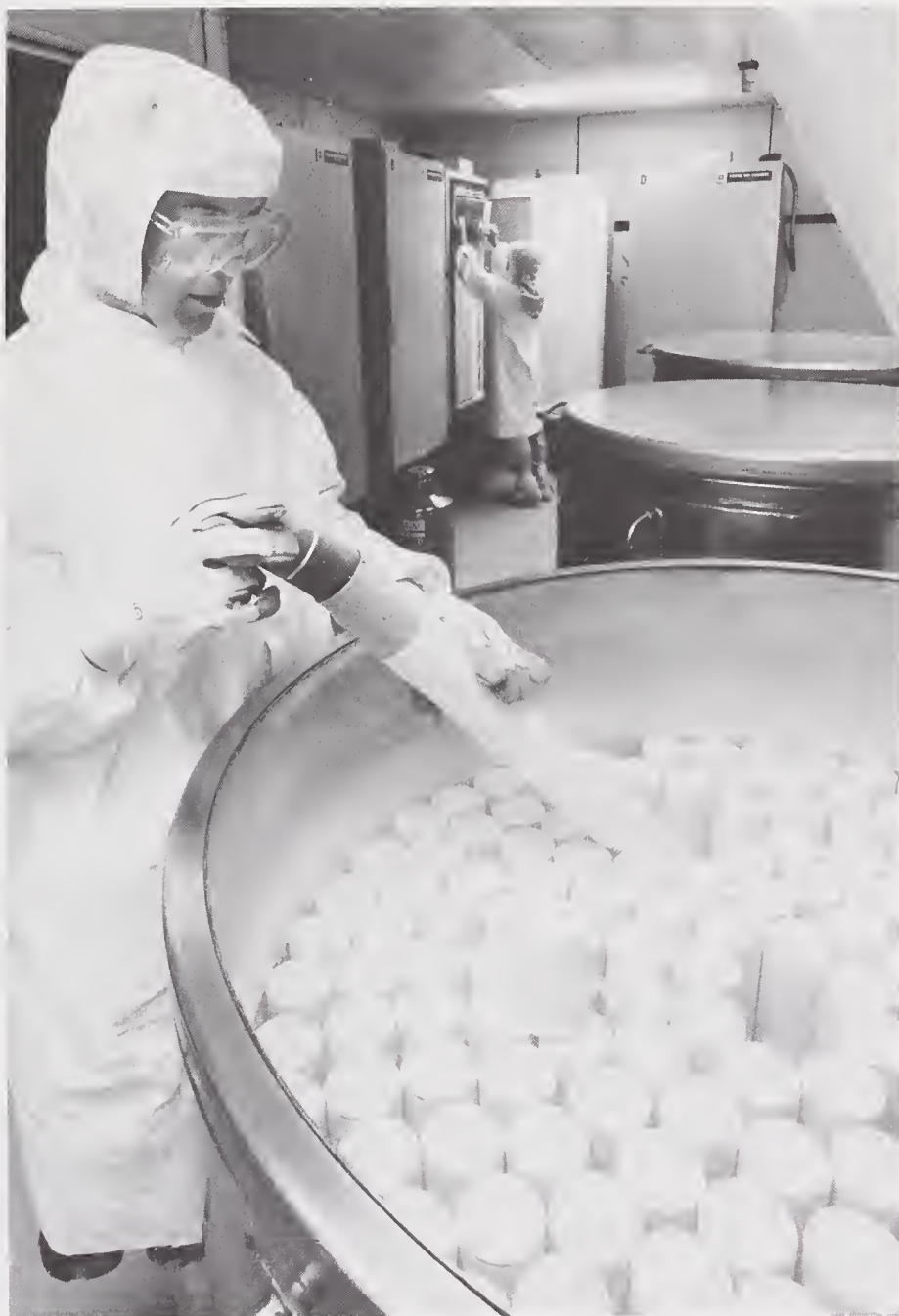
Sally Harrison stores biological samples in a liquid nitrogen freezer as part of the joint NBS/EPA Pilot Environmental Specimen Bank program.
