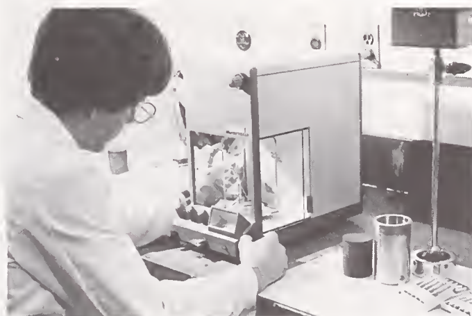
Kevin Rutledge analyzes SRM 1817, Catalyst Package for Lubricant Oxidation. This SRM evaluates the oxidation stability of lubricating oils, i.e. automotive crankcase lubricants. SRM 1817 stimulates the chemical environment in an operating engine, specifically under the ASTM sequence IIID engine test conditions.
