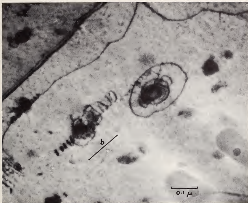
FIGURE 10. Orowan loops around alumina particles in a Cu—30 percent Zn alloy.
