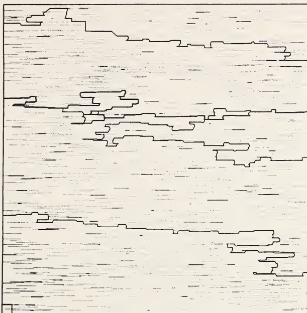
FIGURE 5(b). Diagram obtained directly from the computer by a Stromberg-Carlson 4060 graft plotter for the movement of a "screw" dislocation through an array of linear obstacles of length s . The dislocation moves from the bottom of the array and its position is shown for successive stress increments. The straight parts of the dislocation at the top are non-equilibrium positions which occurred when the dislocation broke out of the top of the array. Infinitely hard obstacles s=2D_s .
