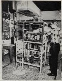
Improved power standards installed during the year included this standard calorimetric wattmeter (left) (page 91). Right: The second ammonia beam spectrometer (maser) was put into operation as part of the Bureau's program to improve its atomic standards of time and frequency (page 89).
