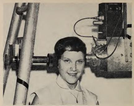
Absolute measurement of the threshold of hearing by bone conduction is expected to be of value in the diagnosis of the nature of certain hearing losses (page 40).
