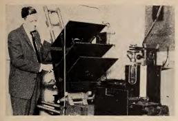
Diagram (right) of equipment used to recalibrate the national candlepower standards against the primary standard of brightness, a blackbody radiator maintained at the temperature of freezing gold (1,063° C). The photometric receiver used to make the comparison is shown above (page 16).
