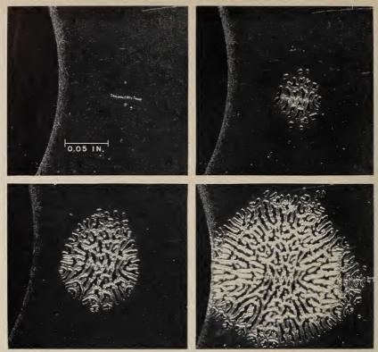
Transparent tape applied to the surface of a metal specimen in which a minute fatigue crack has been induced demonstrates a new effect. As continued cyclic stress is applied, gas evolves in increasing amounts under the tape. The origin of the gas is now being investigated in an effort to shed new light on the processes of metal failure (page 57).
