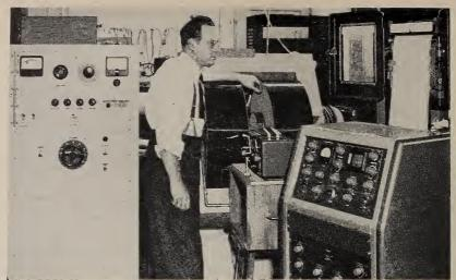
Nuclear magnetic resonance offers a tool for the investigation of the solid state. A study of the absorption of energy by atomic nuclei in solids provides a better understanding of the local electric and magnetic fields that the nuclei experience (page 30).
