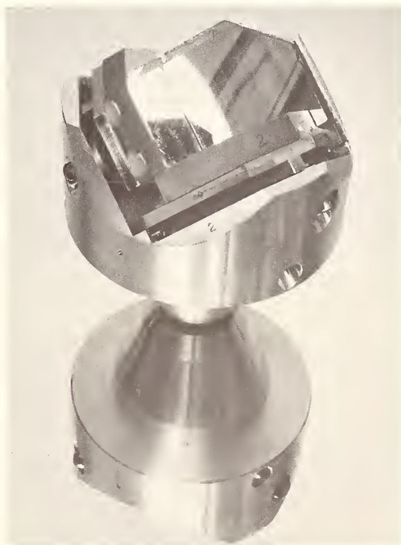
FIGURE 4. The corner-reflector resting on a mirror to show launching and catching surfaces.
