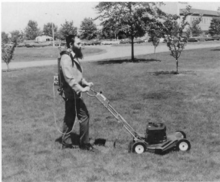
In a project undertaken with the Consumer Product Safety Commission, Jonathan Adler of the NBS Sound Section measured the sound level and thus the hearing-damage potential of a power lawnmower. The sound of the mower was picked up by microphone just below his right ear.
