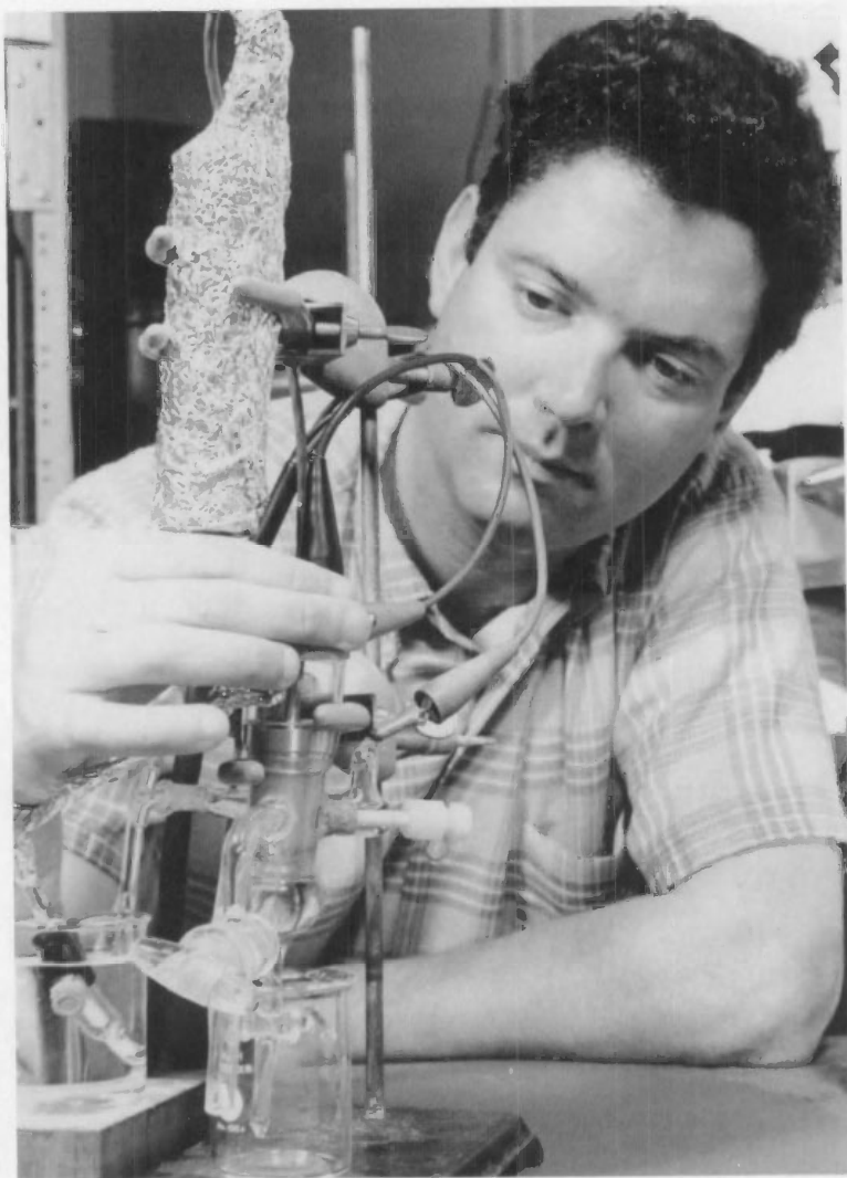
NBS chemist John R. Ambrose developed tests to predict how surgically implanted materials would react to bodily tissues and fluids. In this photograph, Ambrose worked on a laboratory method that simulated crevice-corrosion in the body.
