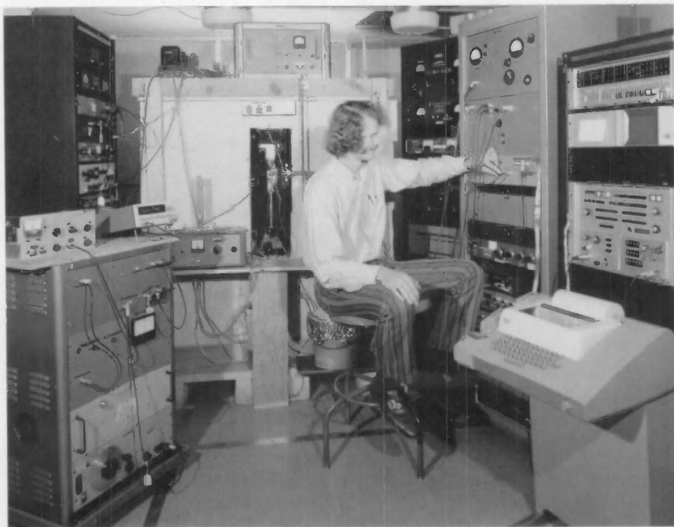
David L. Vanderhart, scientist in the Bureau's Polymers Division, tuned a homemade nuclear magnetic resonance spectrometer in studies of chemical shifts in solids.
