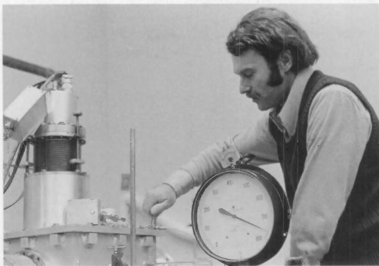
John W. Hastie of the Bureau's Inorganic Materials Division adjusted the pressure in a flame-sampling mass spectrometer prior to observation of species involved in flame inhibition.
