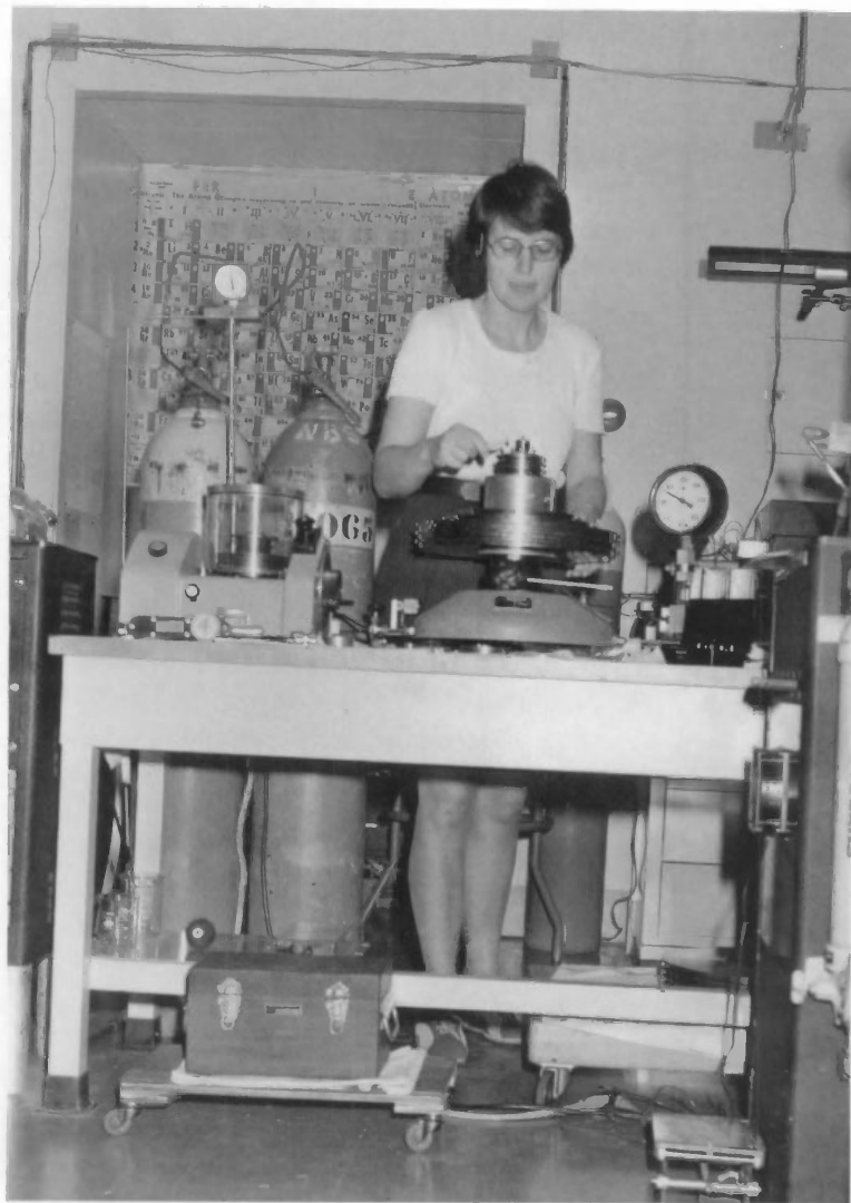
Johanna M. H. L. Sengers adjusted the load on a piston gage which was used for accurate measurement of the pressure of gases used in her studies of critical phenomena.
