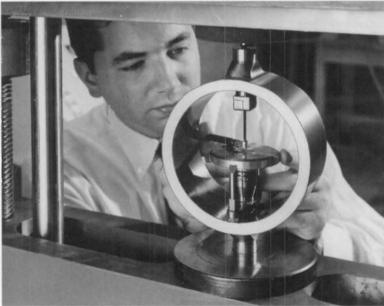
Arnold J. Mallinger inspected a proving ring before its calibration as a force standard in a deadweight machine at the National Bureau of Standards.
