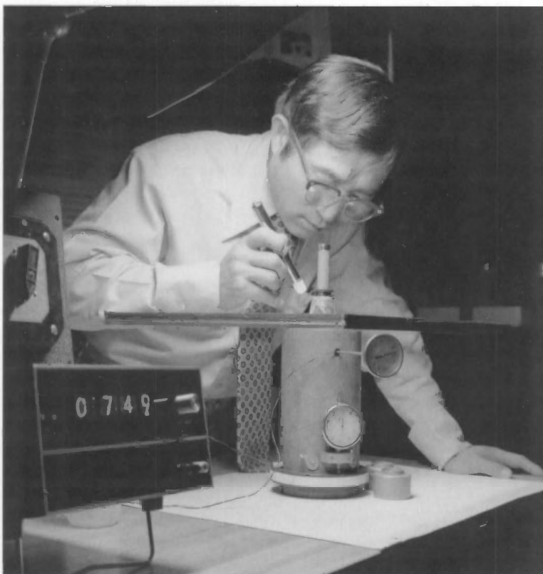
Mahn Hee Hahn, Research Associate from the American Society for Testing and Materials, with the dew/frost point apparatus he developed to measure the moisture content of the air space in sealed insulating glass. The device received the IR-100 award from Industrial Research magazine as one of the most significant new technical products of 1975.
