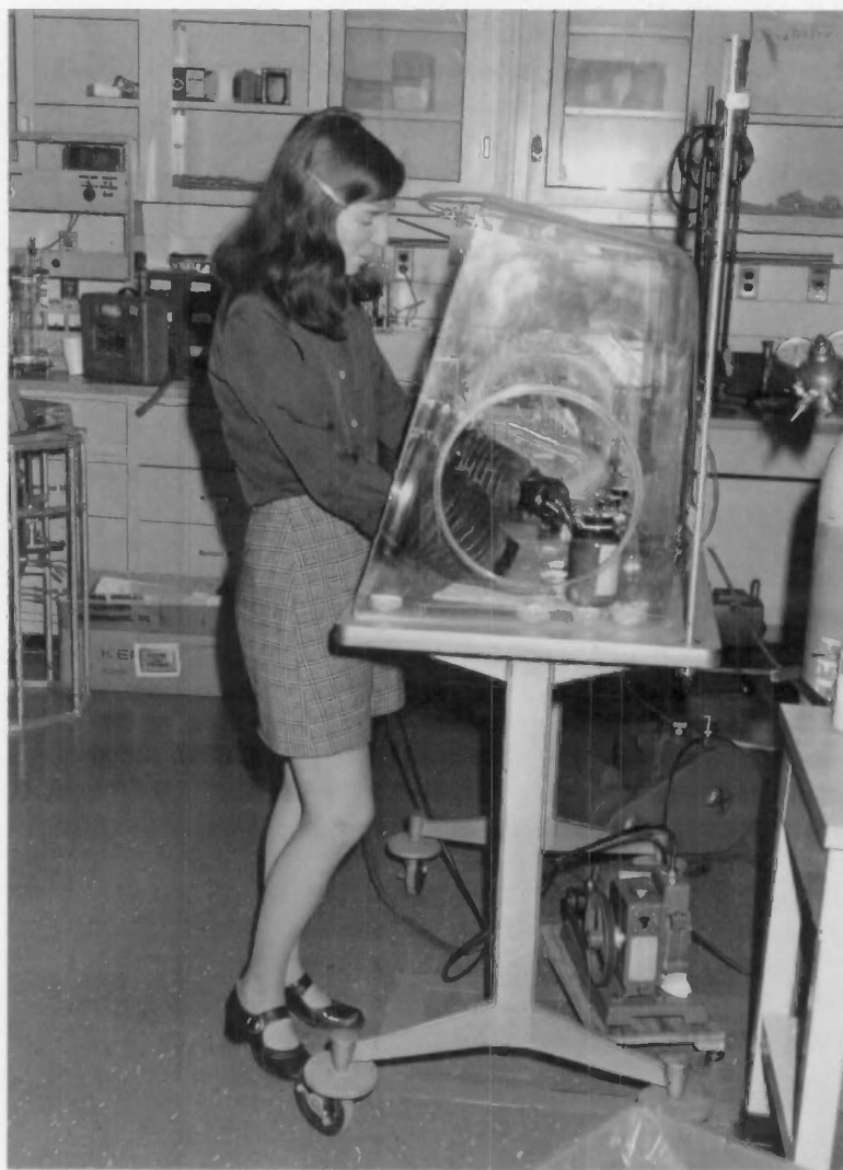
Sandra C. Greer mixed nitroethane and 3-methylpentane in a dry box as part of her research on critical phenomena in binary liquid mixtures.
