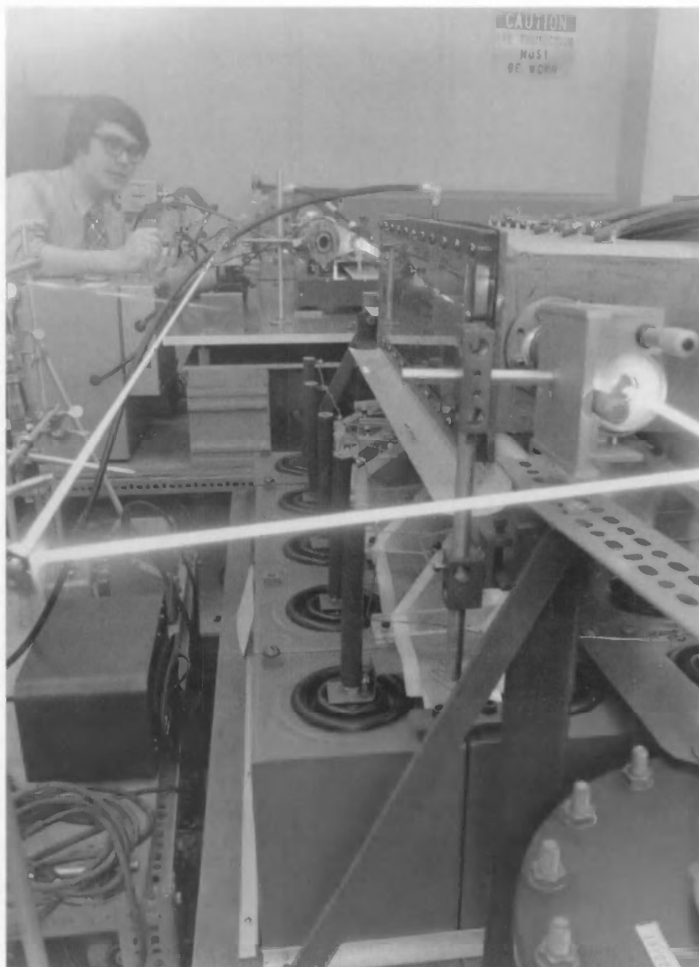
George H. Atkinson used a dye laser to detect free radicals, a technique that he developed at the National Bureau of Standards with Allan H. Laufer and Michael J. Kurylo.
