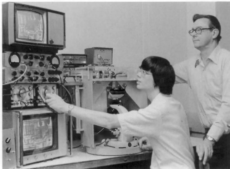
David W. Berning (left), an electronics engineer, and David E. Sawyer, a physicist, of the NBS Electronic Technology Division, operated the laser flying-spot scanner they developed for testing semiconductor devices.
