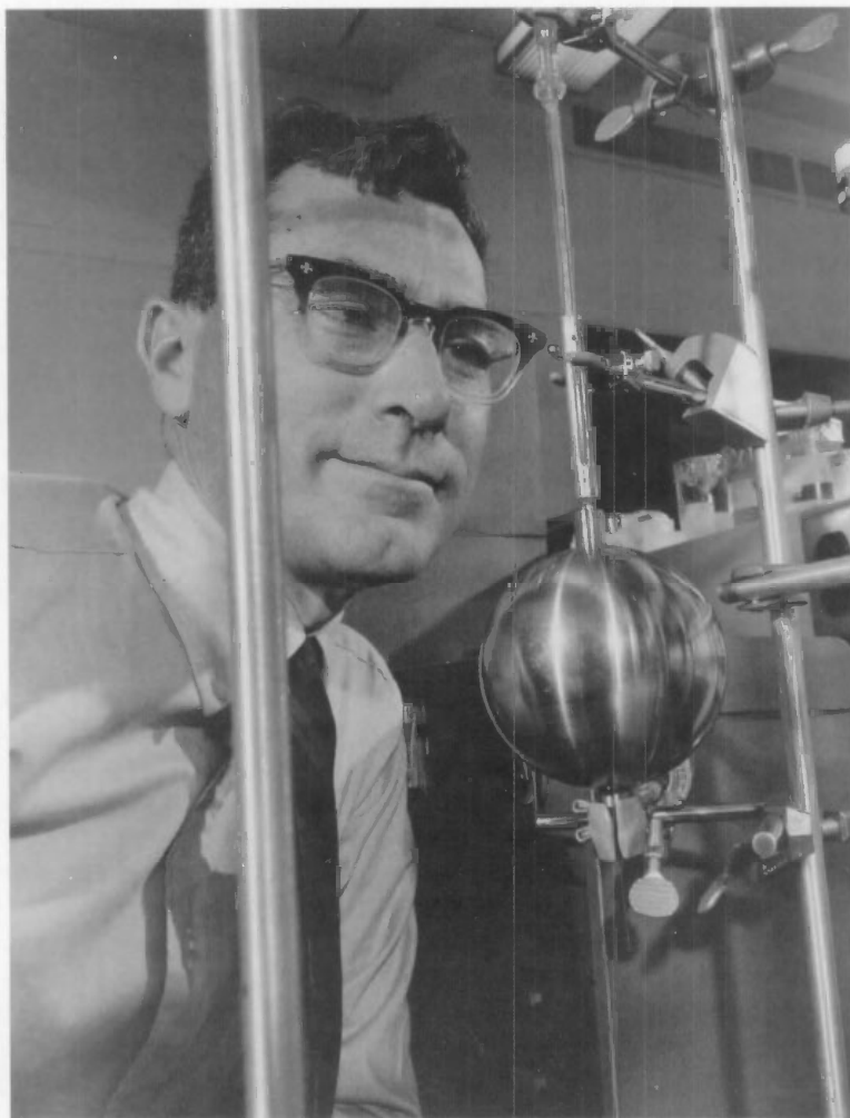
Elliot Kearsley inspected the height of the liquid inside a hollow sphere that, when excited, became a rotational pendulum, turning first in one direction and then in the other. It could be used to make absolute viscosity measurements, the viscosity of the sample liquid being calculated from observed parameters, including the period of oscillation.
