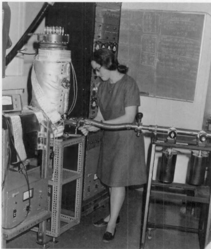
Margaret G. Scroger connected an absorption roughing-pump system to a high-vacuum oven used in refractory-metal thermocouple research.
