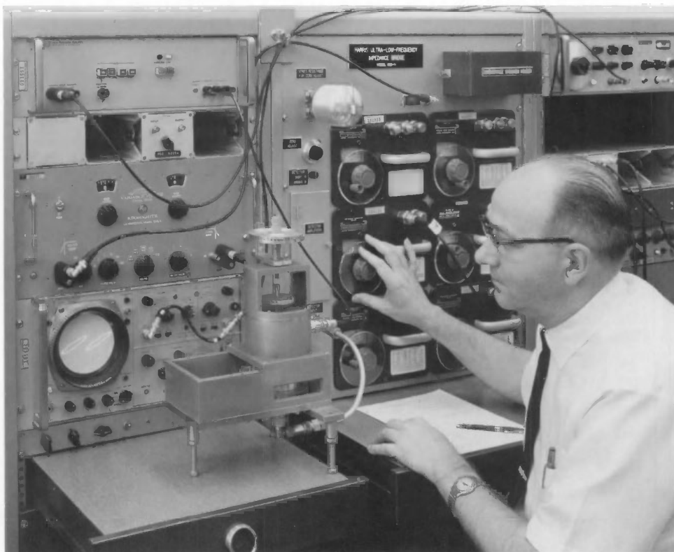
William P. Harris of the National Bureau of Standards made dielectric measurements on a specimen with an NBS-constructed ultralow-frequency bridge. Such measurements were important for determining the suitability of materials for electrical insulation and for molecular behavior studies.
