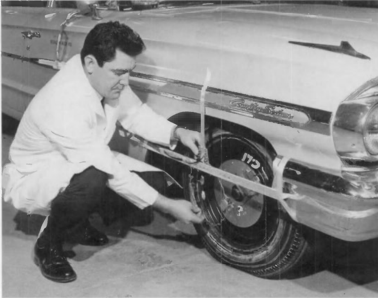
As part of a 1968 research project, Glenn Ludwig of the NBS Office of Vehicle Systems Research (OVSR) adjusted an antenna for picking up a telemetry signal indicating tire temperature. The instrumentation was used to study tire performance under an automobile safety program conducted by OVSR for the Department of Transportation's National Highway Safety Bureau.
