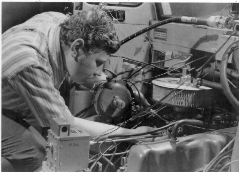
NBS scientists compared the performance and exhaust emission characteristics of motor vehicles run on gasoline, compressed natural gas, and liquefied petroleum gas for the U. S. Postal Service. In this photograph, David K. Ward made engine adjustments during a test on a half-ton truck.
