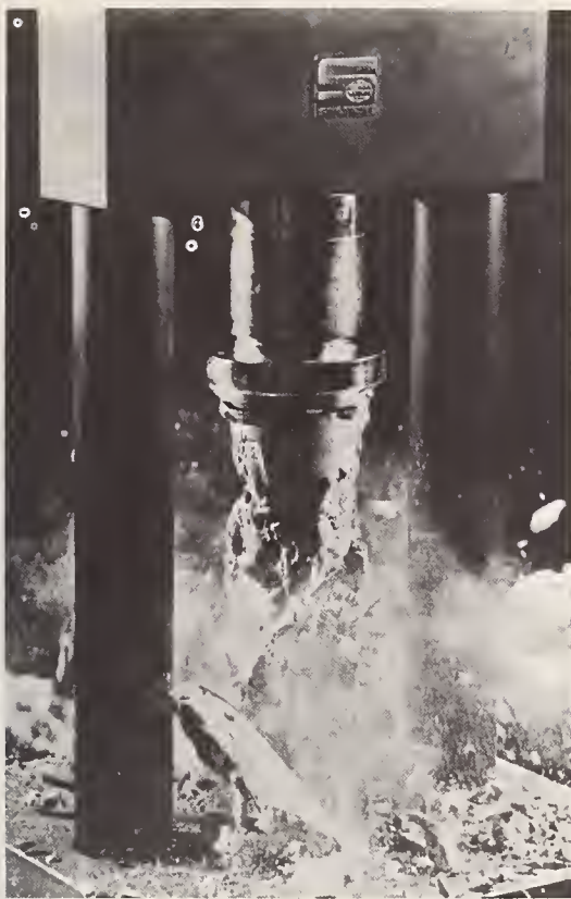
FIGURE 23. Explosive failure of standard concrete cylinder specimen in compression test by Soiltest, Inc.
