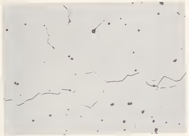
FIGURE 13. Crack propagating through polycrystalline Al_2O_3 . Note the random nature of the crack path. After R. L. Coble, ref. [14], p. 623.
