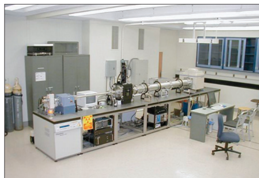
Figure 2. The world's first laboratory scale CD-SAXS prototype constructed on the NIST campus. Shown is the rotating anode molybdenum source (left side) used to generate high energy X-rays for transmission measurements on samples measured at varying angles of incidence on a 2-dimensional detector (back right).
