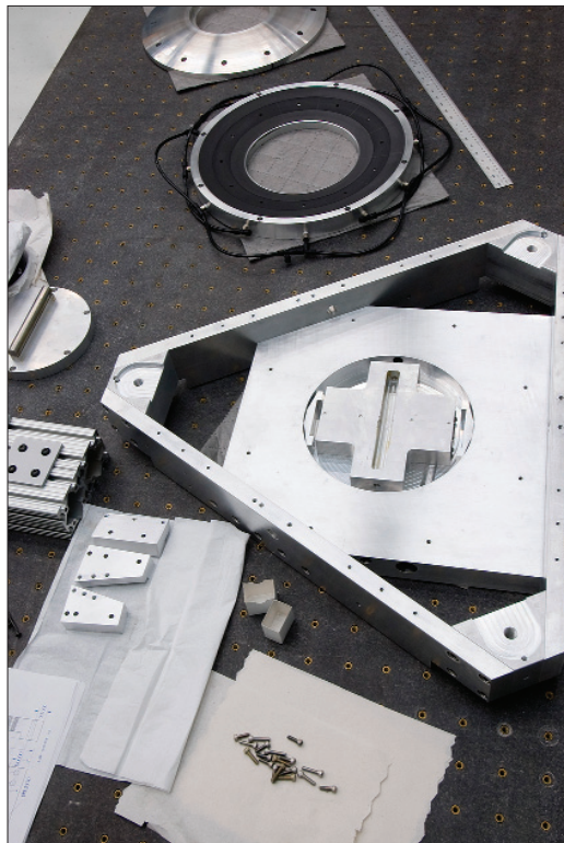
Figure 5. Spherical air bearing for CDPBD goniometer, seen during assembly. Spherical male/female components with 0.7 m radius of curvature for goniometer tilt (top), and kinematic air bearing assembly for goniometer translation (center, right).
