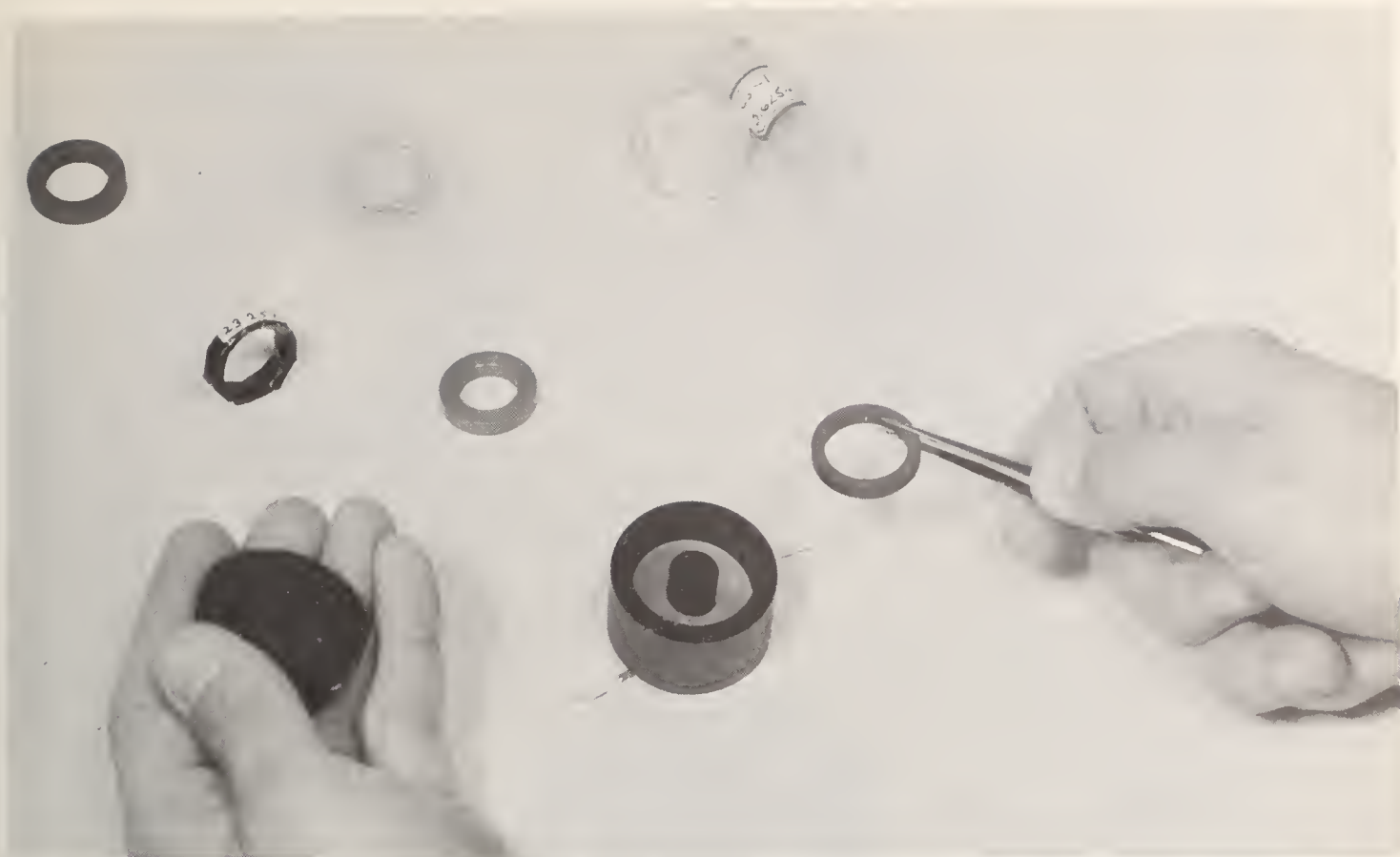
Figure 3. RF Permittimeter. (The walls, end plates and center conductor of the coaxial structure are made of ferrite. A primary winding excites the circular electric field about the center post. Toroidal dielectric or conductivity substances are inserted in this field for evaluation. A toroidal plastic container with a channel in which liquids can be placed provides measurements on the dielectric or conductivity properties of fluid substances).
