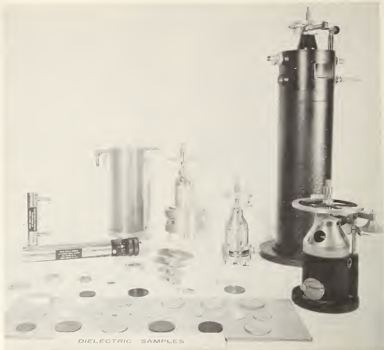
Figure 1. Representative Dielectric Electrode Systems Used at NBSBL. (Tall structure to the right is a coaxial variable length re-entrant cavity).
