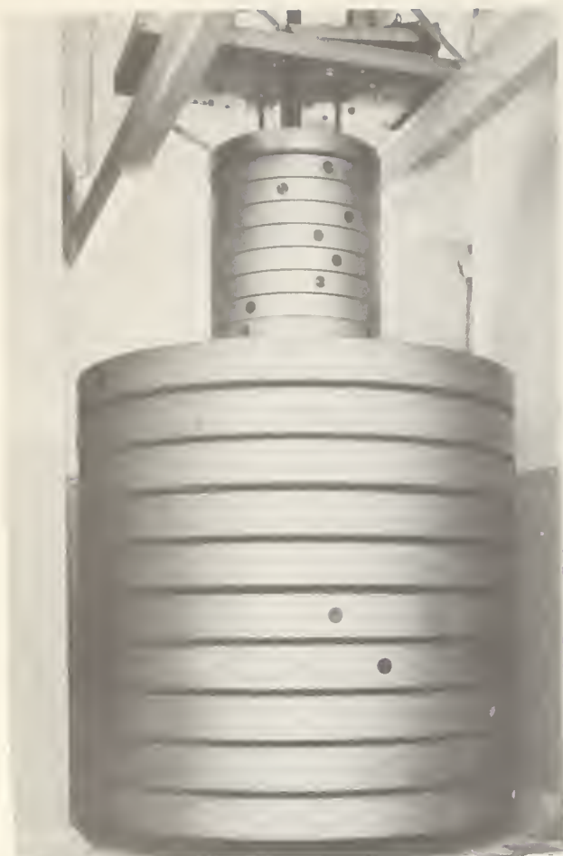
Figure 9. Weights and lower part of the 111,000-lb capacity dead-weight machine.
