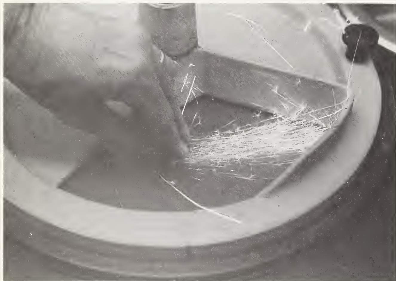
Solid metal SRM's are re-surfaced as needed for optical emission spectroscopy.
