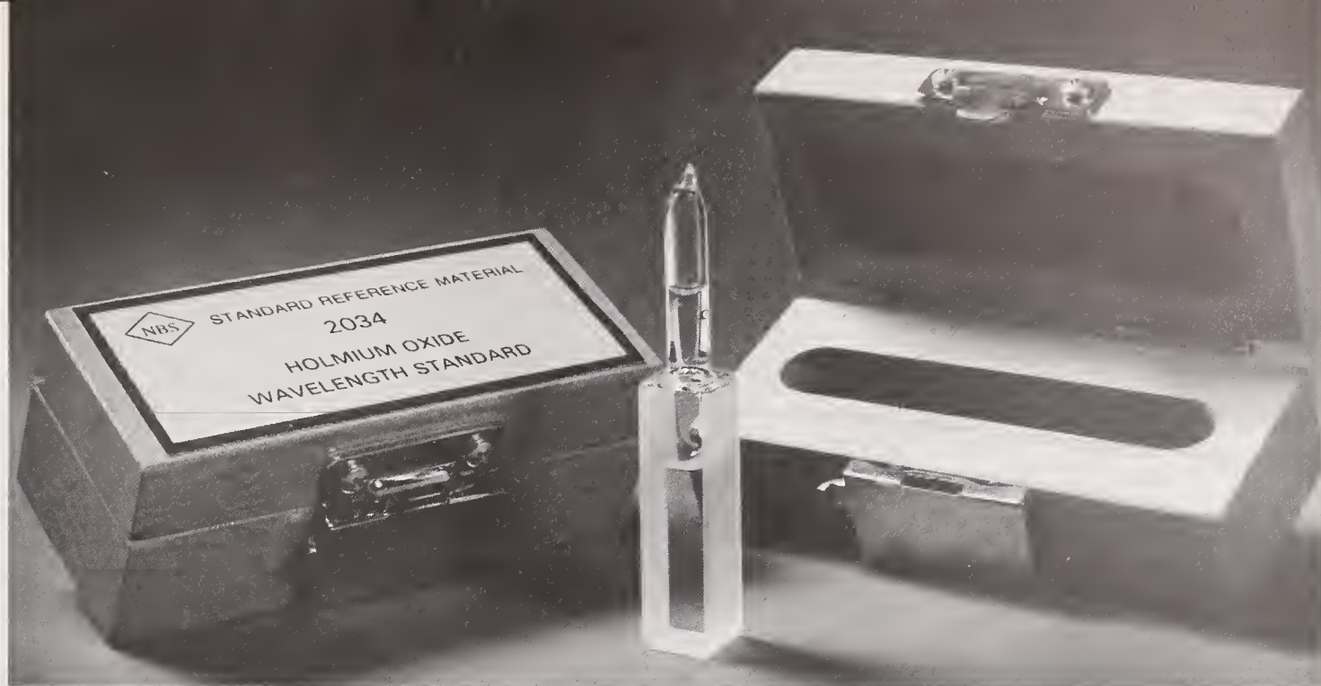
SRM 2034 is 4% holmium oxide in 10% perchloric acid in water, sealed in a non-fluorescent, fused-silica cuvette for use as a spectrophotometric wavelength SRM.
