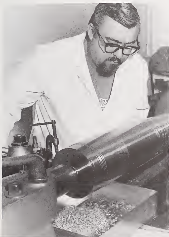
Frank Mills controls the chipping of a titanium alloy that will be ground, sieved, and blended to insure high homogeneity before analytical testing for certification.
