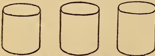
FIG. 5. RELATIVE SIZE OF AVOIRDUPOIS OUNCE, 30-GRAM, AND TROY OUNCE (BRASS) WEIGHTS. (ACTUAL SIZE.)
