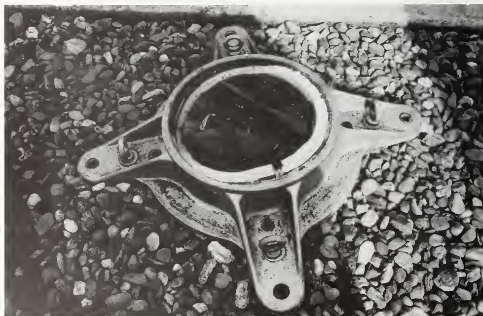
Figure 5.4.23 Porcelain failed at the base plate of this current-voltage transformer.
