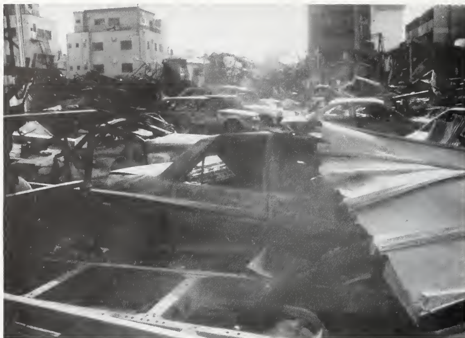
Figure 6.2.11 Parking area where automobiles contributed to fire spread between buildings.
