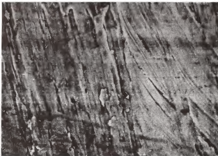
Figure 76. SEM picture of a copper surface preheated to 700°C. Magnification: 2000X
