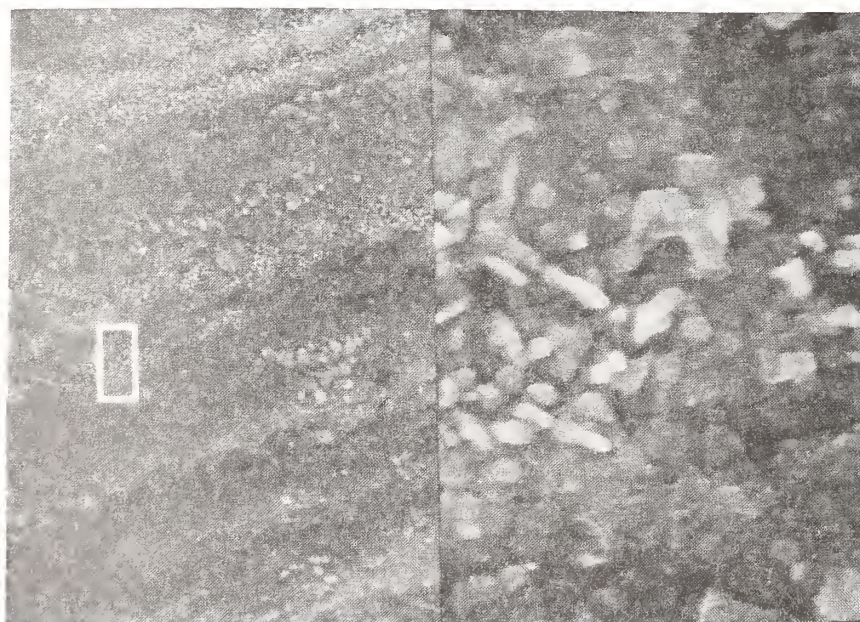
Figure 31. SEM photograph of a deposit 61 \mu\text{g}/\text{cm}^2 on an iron wire surface for 2 seconds with 1.55% TCP at 700^\circ\text{C} . Magnification is 1000X on the left frame. The square window on the left frame is magnified 10 times and shown on the right frame. Each marker represents the length on its frame.
