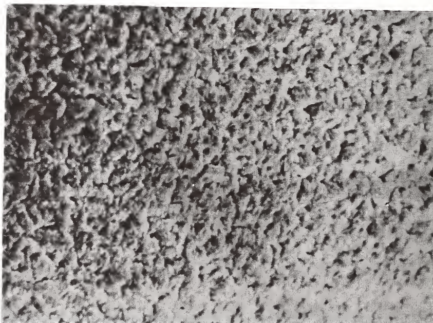
Figure 77. SEM picture of a deposit ( 173 \text{ ug/cm}^2 ) on a copper surface. 1.0% TMPH in air, 700°C. Magnification: 2000X
