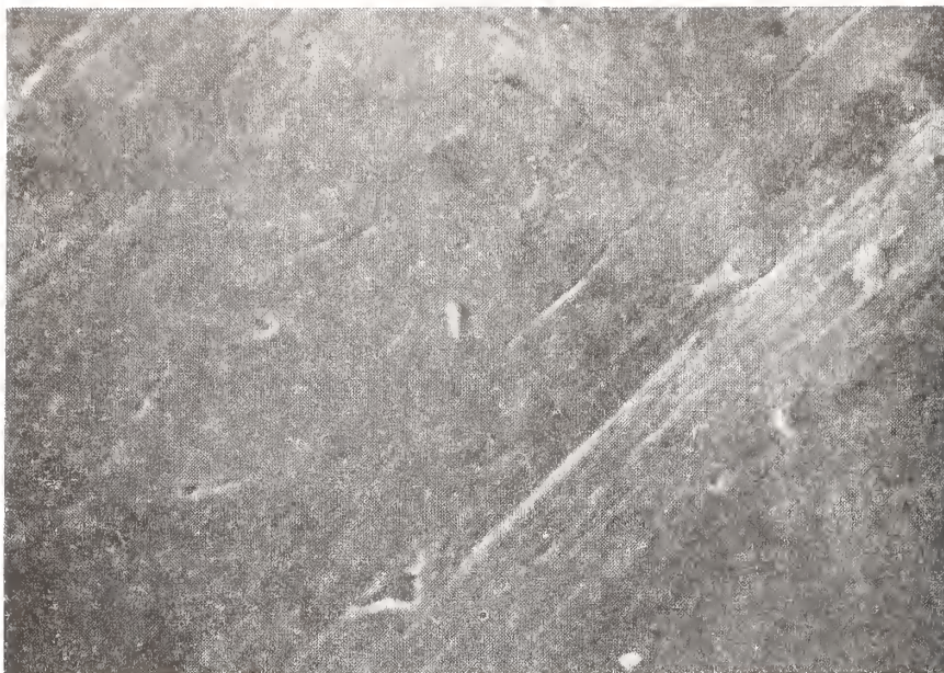
Figure 64. SEM picture of a stainless steel surface, preheated to 700°C. Magnification: 2000X
