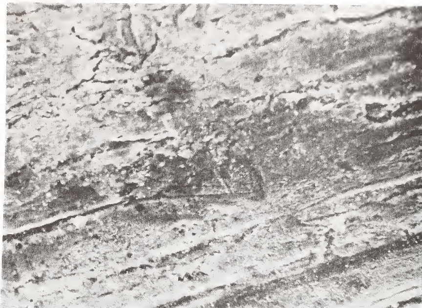
Figure 72. SEM picture of an iron surface preheated to 700°C. Magnification: 2000X
