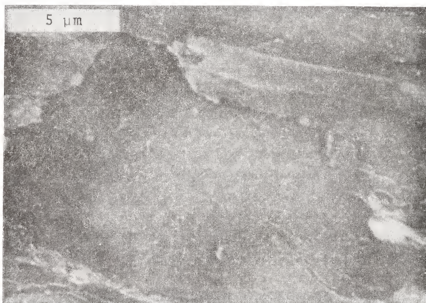
Figure 44. EDAX illuminated area of a cracked chip (backside) from TCP deposit on iron wire. Magnification is 5700X.
