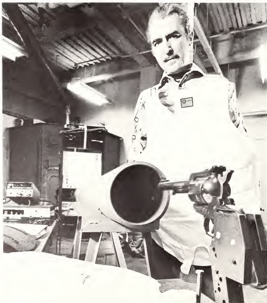
The Bureau's Law Enforcement Standards Laboratory develops standards and guidelines for law enforcement and criminal justice equipment. Ralph Gorden is shown with laboratory arrangement used to test performance of body armor worn by police officers.
