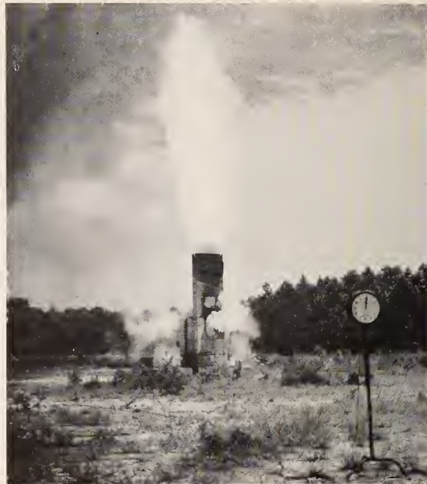
FIGURE 11. Discharge of flames about 60 ft above vertical vent after vent cover blown off, experiment 11 in Beltsville vault.
