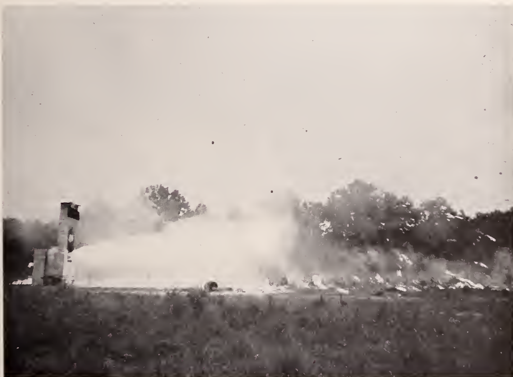
FIGURE 14. Violent discharge of flames, film cans, and film from horizontal vent during experiment 12.
