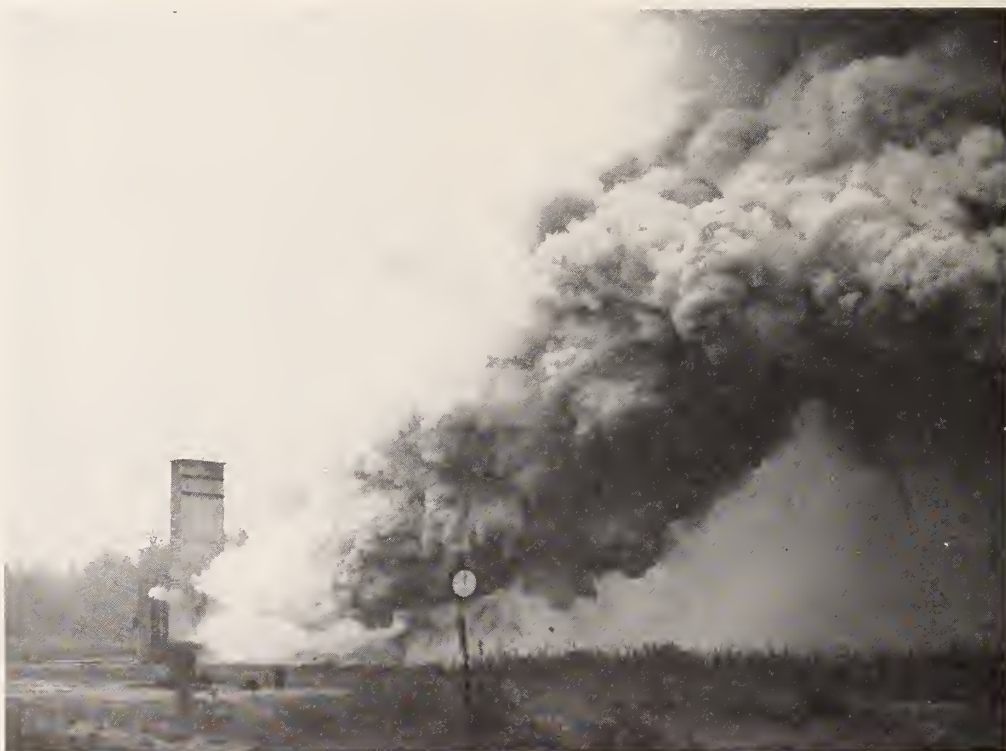
FIGURE 12. Discharge of very dense fumes from horizontal vent just as ignition of fumes initiated at vent, experiment 9.
