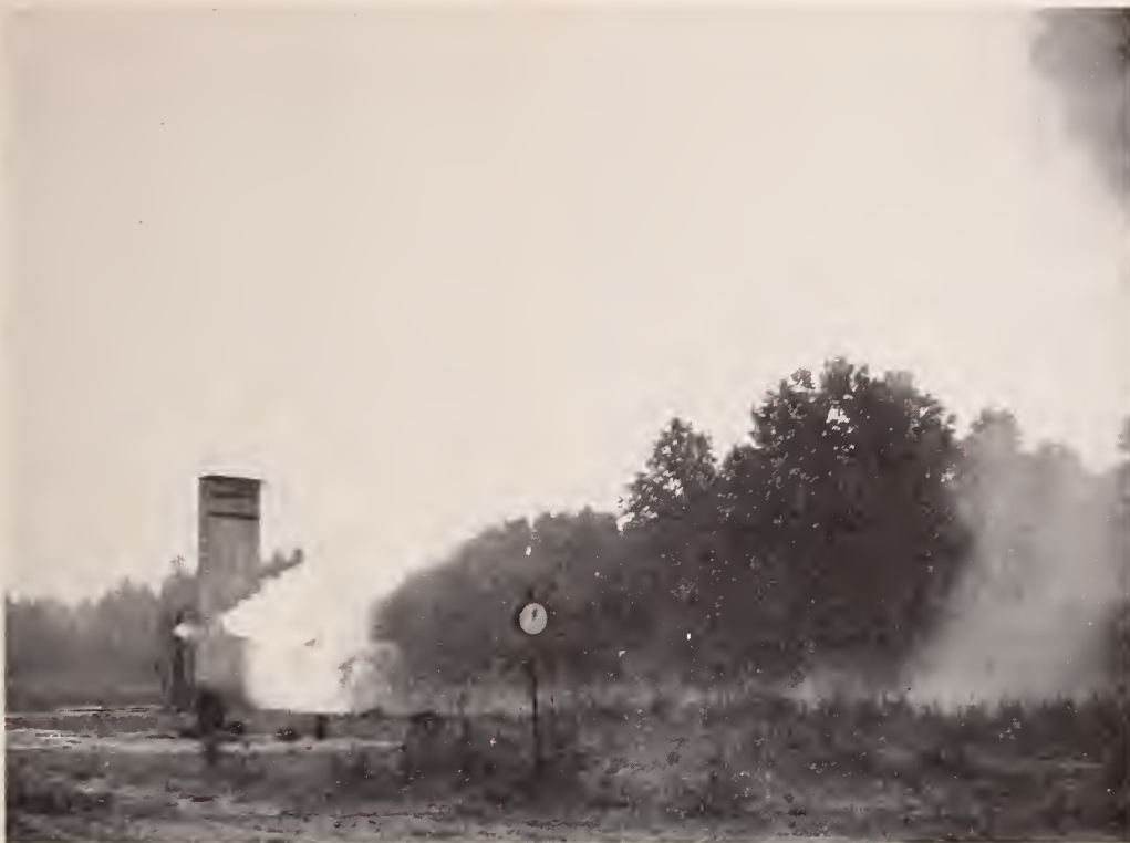
FIGURE 13. Appearance during experiment 9 about 10 sec after that in figure 11, showing that dense fumes were almost completely burned.
