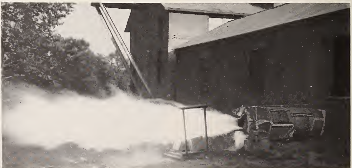
FIGURE 8. Discharge of gas and flames from 22-ft 3 steel chamber during experiment 8 at National Bureau of Standards.
