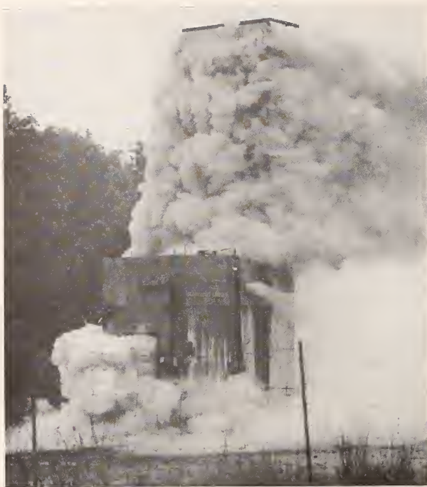
FIGURE 10. Discharge of dense fumes from Beltsville vault during experiment 2, vent cover in place on vertical vent.
