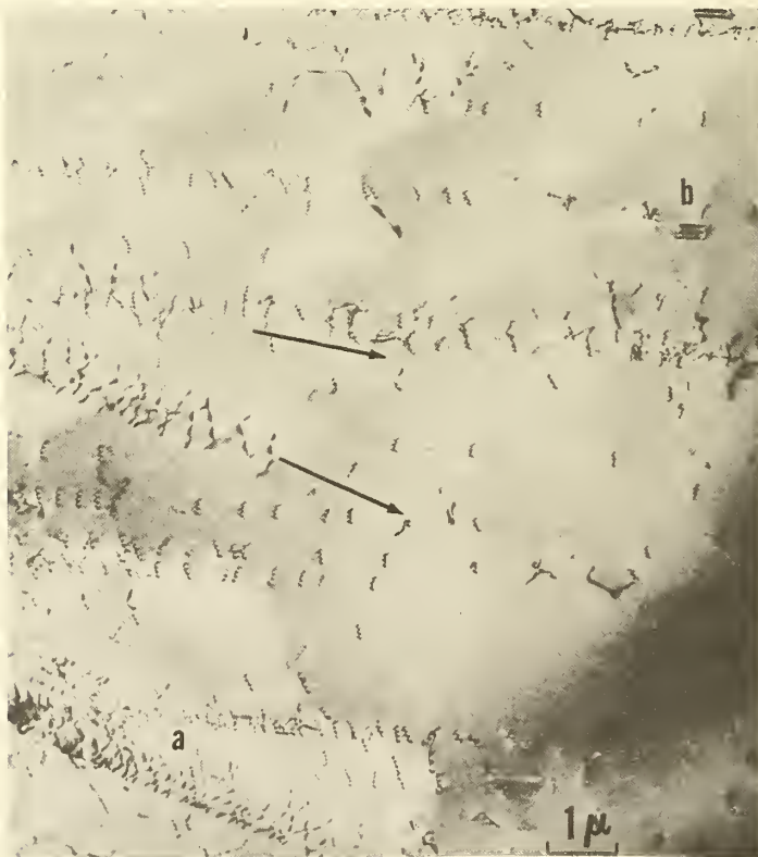
Figure 44. 310 stainless steel strained \sim 3\% . Arrows indicate slip systems; (a) are dislocation interactions at dislocation pile-up where two slip planes intersect and (b) is a stacking fault separating two partial dislocations. 40,000X
