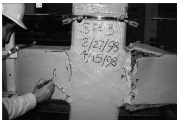
Figure 5–2 Retrofitted beam-column connection after testing (Mosallam, 2000)
