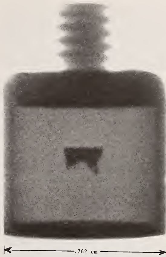
Figure 2. X-ray of ^{252}\text{Cf} fission neutron source. Californium deposit is at the center of the cylindrical capsule.
