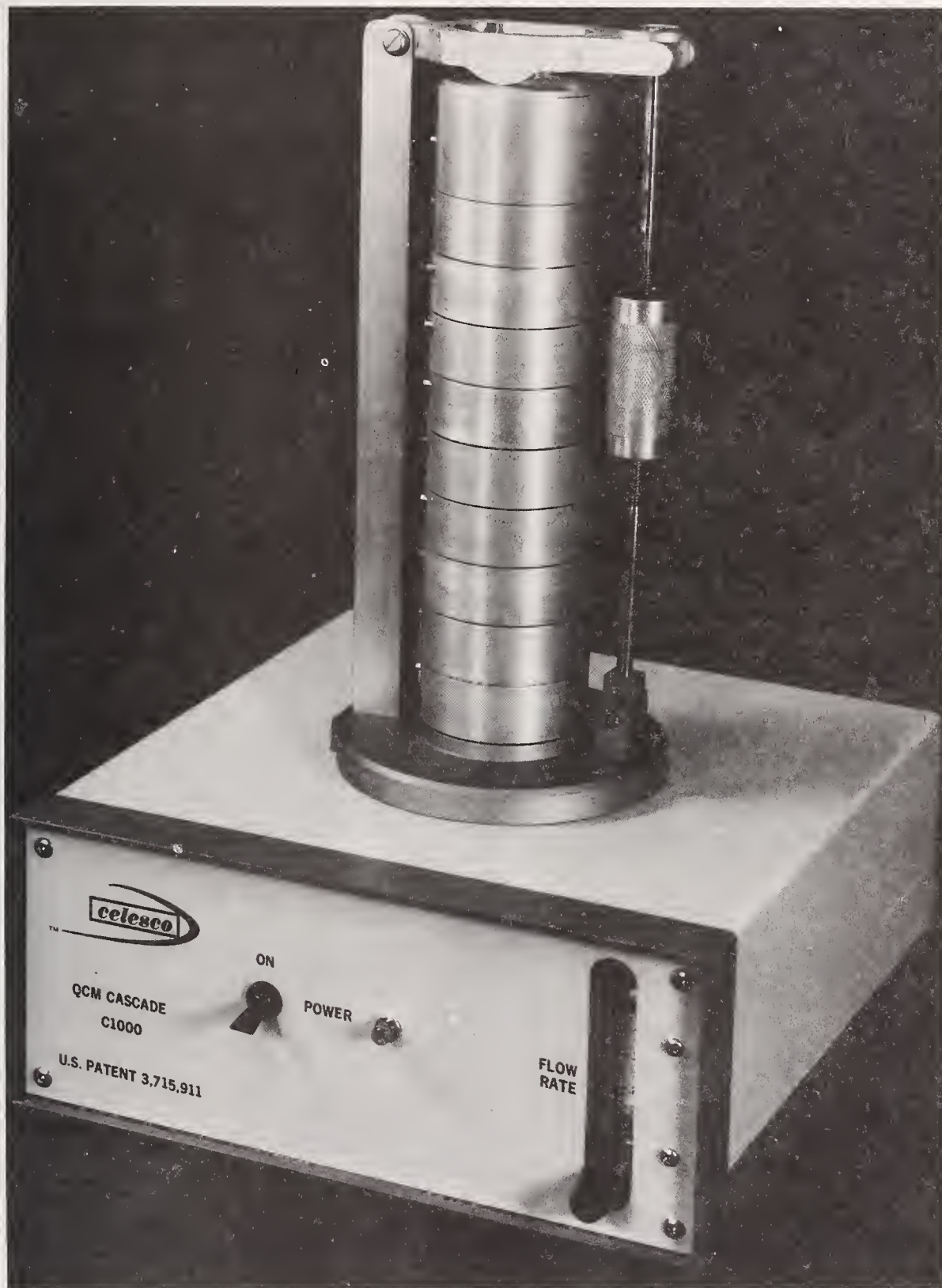
Figure 5. Ten stage QCM cascade.
