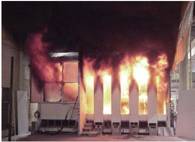
BFRL measured the thermal behavior of gypsum/steel wall assemblies subjected to severe fire conditions.
