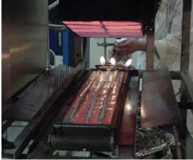
Methane-fired panel which creates a flux gradient for flame spread test of extruded flame retardant polymer sample rods.
