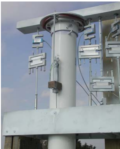
State of the art field exposure apparatus for naturally stressing sealant samples is positioned on BFR's roof. Numerous physical and environmental variables are being monitored on a continuous basis. Physical properties include stress and strain within the sealant while environmental variables include sealant temperature and moisture content.
