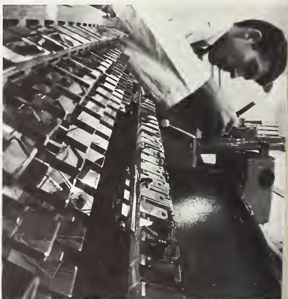
Gage blocks, checked by NBS, are fundamental length measuring tools on American production lines.
