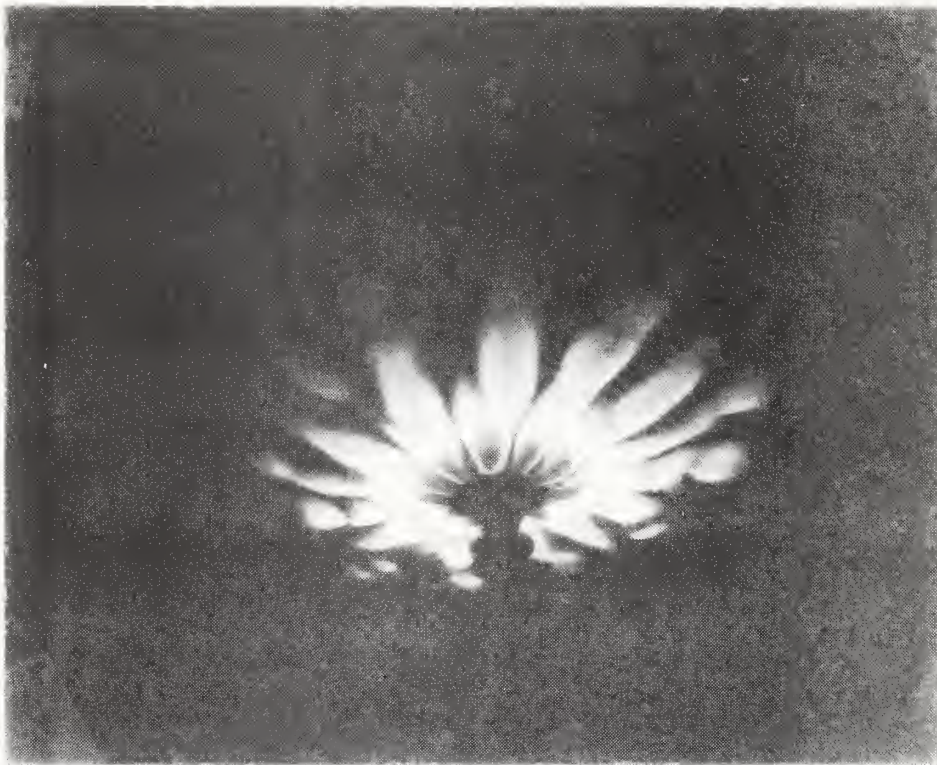
Fig. 8. Swinging daisy flower of a propane flame with H = 2.0 mm and Q = 7.6 kW (1/60 s exposure).
