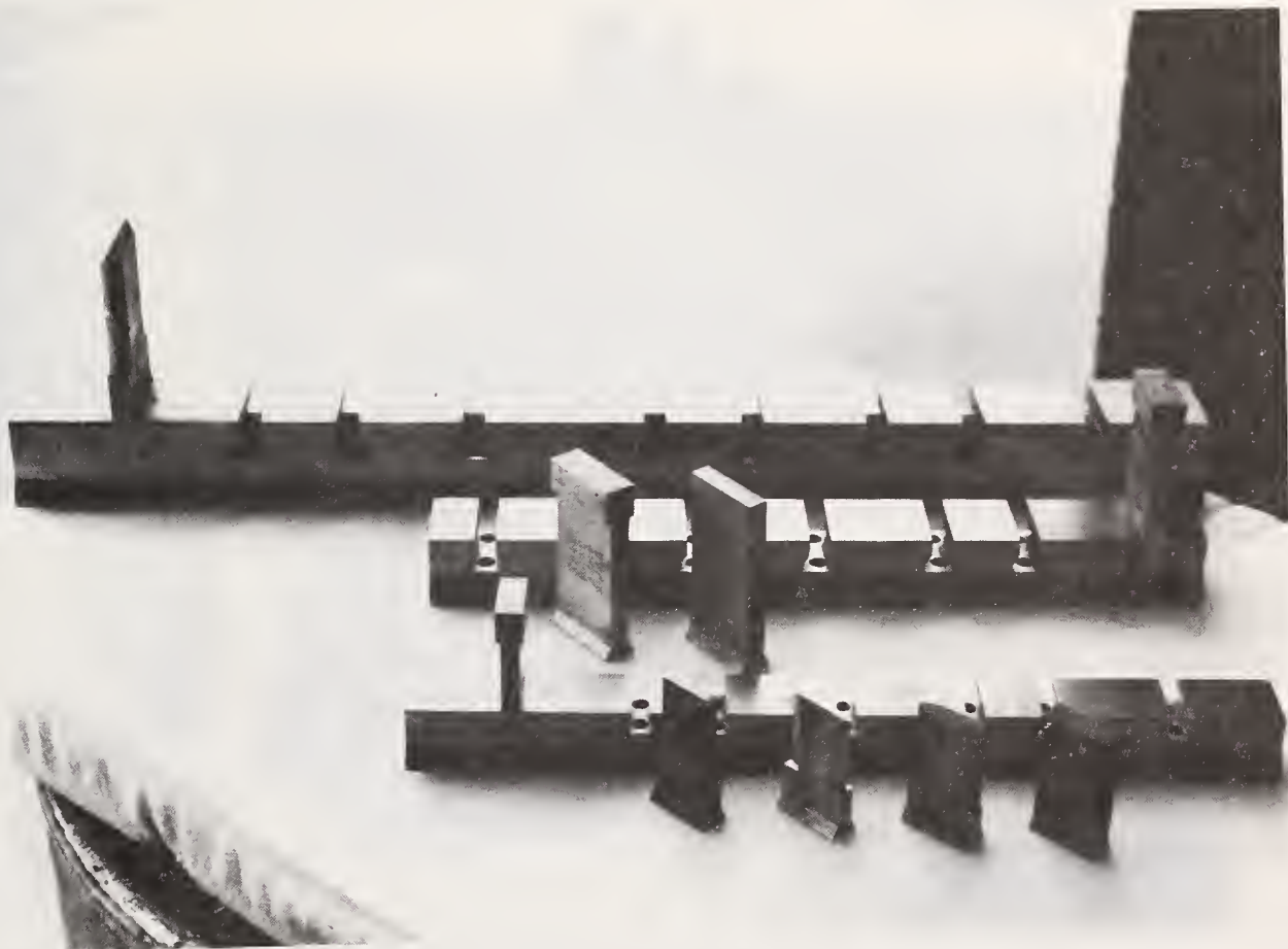
Figure 4: The Knife bar and the different types of hammers used.
