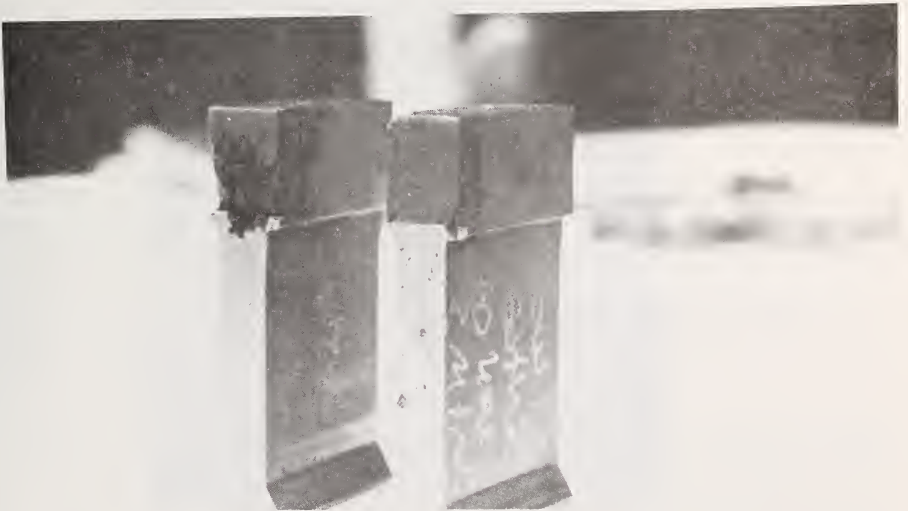
Figure 16 : Failure of the hammers with carbide insert.
