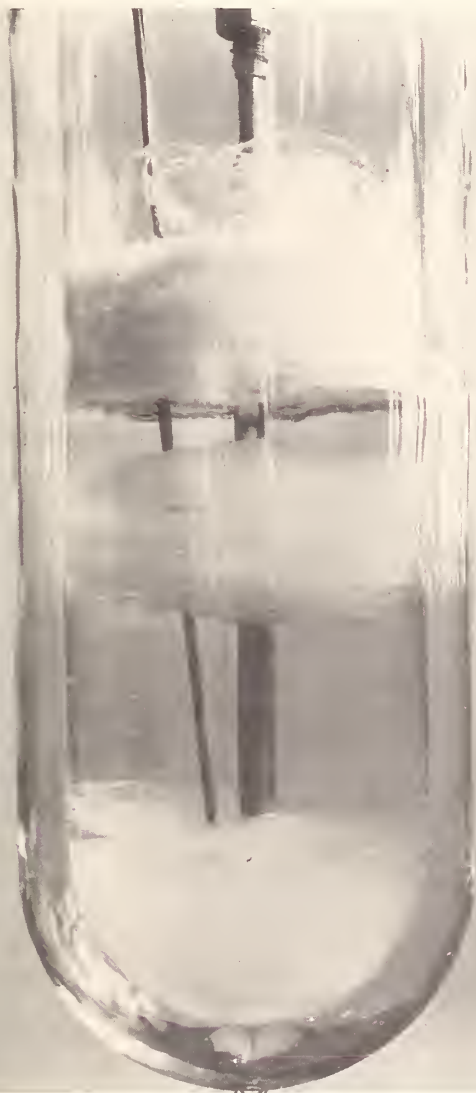
Slush hydrogen is formed at the bottom of a flask at the NBS cryogenics laboratory in Boulder, Colo. Solid hydrogen, formed on the surface of liquid hydrogen, sinks to the bottom and breaks into very fine particles.
