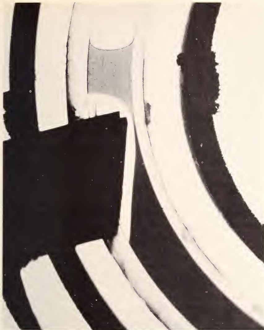
Close-up view of the NBS apparatus used to obtain ultrapure materials. One impurity in the substance is a red dye which shows as gray in the picture. Two silver strips (left center) are in front and back of a crystallizing mound. Note that the color of material in the mound is lighter than the surrounding liquid because it is rejecting the dye impurity as it crystallizes.
