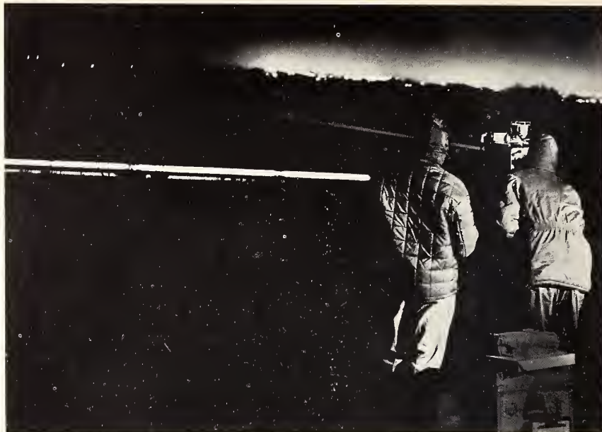
Scientists from NBS and the Coast and Geodetic Survey test a laser-geodimeter over an 8-mile path. The incorporation of a laser as the light source rather than the mercury lamps usually used promises to improve the accuracy and range of the geodimeter.
