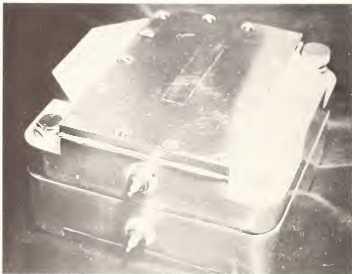
Figure 12. Proportional counter for measuring the number of decays of electron-capture nuclei.
