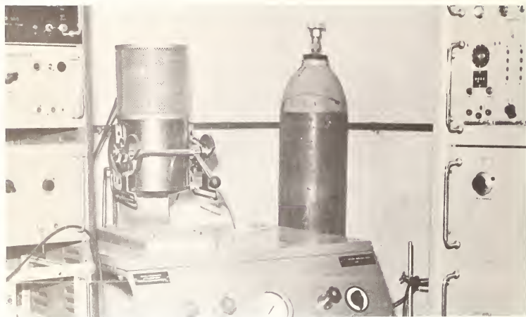
Figure 6. 2\pi alpha-particle ionization chamber.
