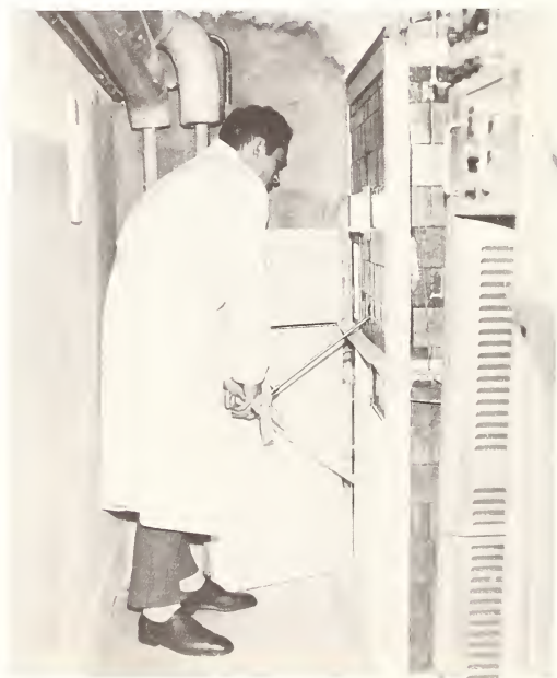
Figure 7. Arrangement for 4\pi integral ionization chamber for relative measurements.
