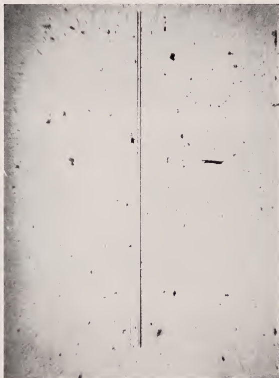
FIGURE 4. Artificial "doublet" caused by nonvertical slit.
