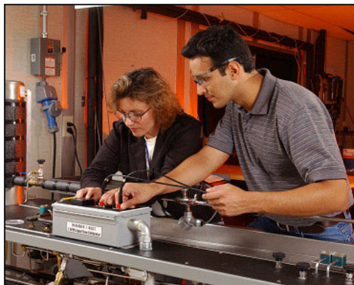
A dual rotor turbine meter is installed in the test section of the 2 L Hydrocarbon Liquid Flow Standard.
