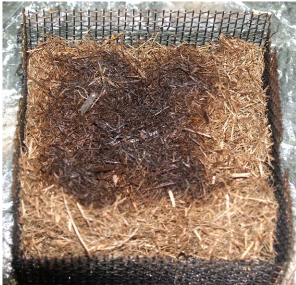
Figure 59. Bottom (left) and top (right) views of a fine Florida grass fuel bed are shown after the fuel was removed from the heated plate held at 290 °C with a low wind applied. Glowing combustion was not observed.
