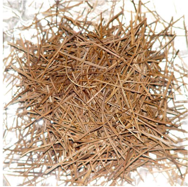
Figure 61. Bottom (left) and top (right) views of a pine needle fuel bed are shown after the fuel was removed from the heated plate held at 290 °C with no wind applied. No glowing combustion was observed.
