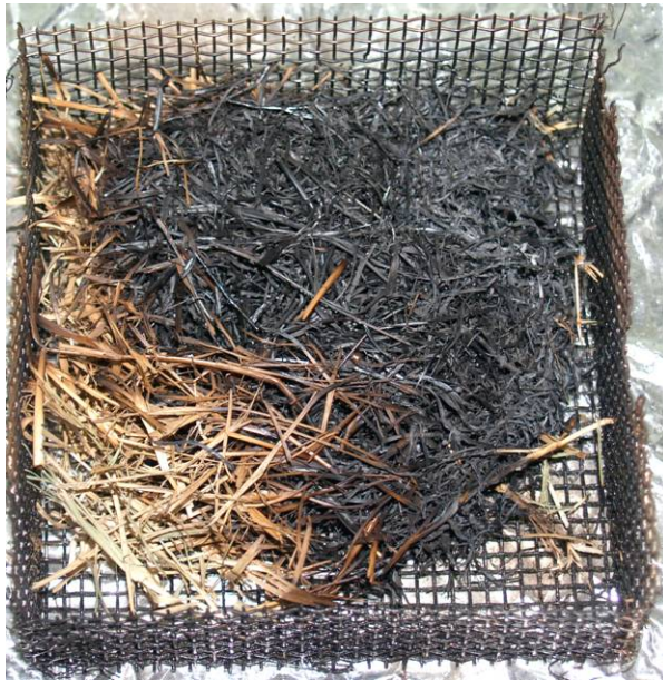
Figure 49. Bottom (left) and top (right) views of an August tall fescue fuel bed are shown after the fuel was removed from the heated plate held at 310 °C with a low wind applied. Glowing combustion and flaming were observed.
