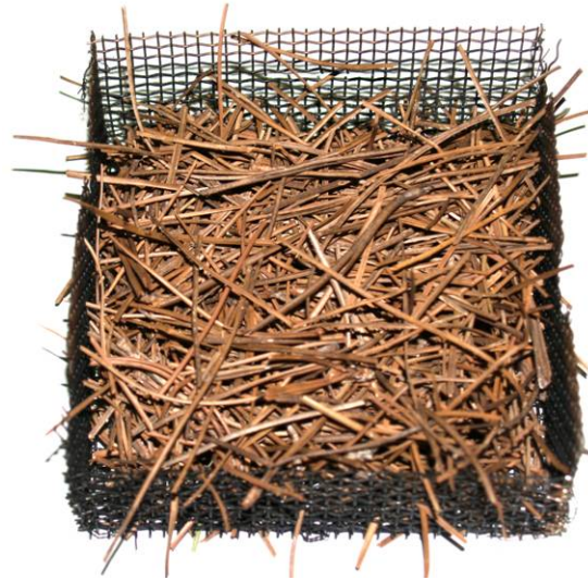
Figure 18. Photograph of pine needles in wire-screen cage.
