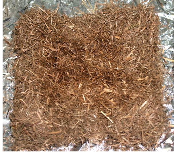
Figure 58. Bottom (left) and top (right) views of a fine Florida grass fuel bed are shown after the fuel was removed from the heated plate held at 310 °C with no wind applied. Glowing combustion was not observed.
