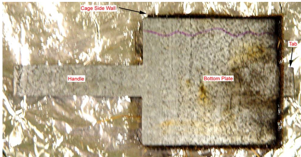
Figure 7. The wire cage with its removable steel-plate bottom in place is shown looking down from above.
