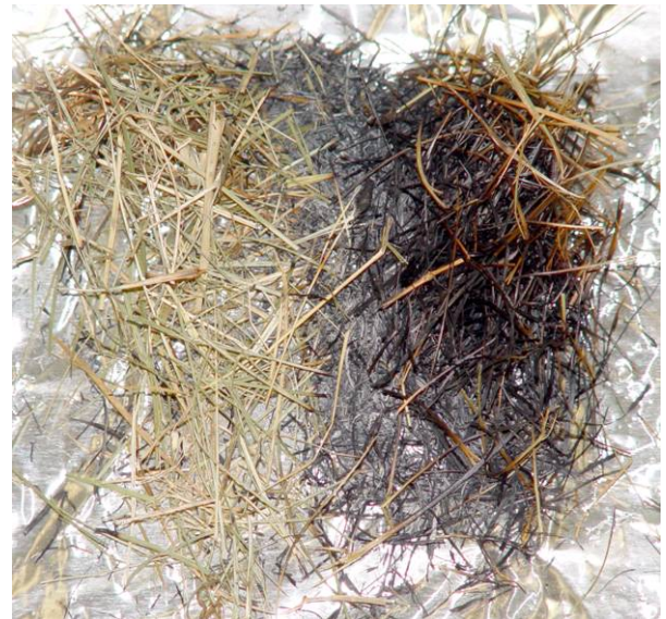
Figure 35. Bottom (left) and top (right) views of a May tall fescue fuel bed are shown after the fuel was removed from the heated plate held at 336 °C with a high wind applied. Glowing combustion was observed after 134 s.
