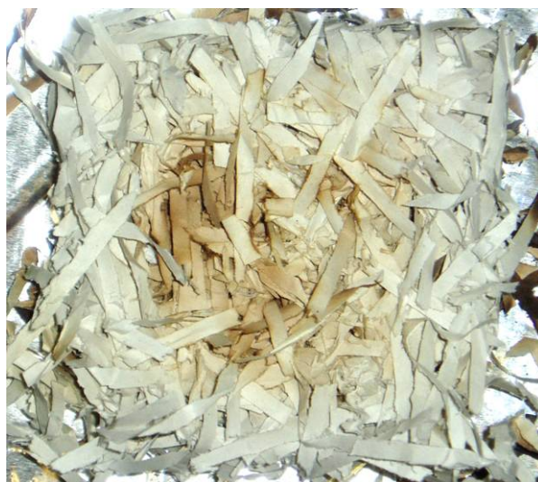
Figure 26. Bottom (left) and top (right) views of a shredded newsprint fuel bed are shown after the fuel was removed from the heated plate held at 332 °C with no wind applied. Glowing combustion was not observed.
