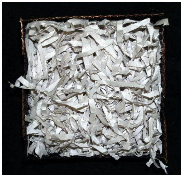
Figure 12. Photograph of shredded newsprint in wire-screen cage.
