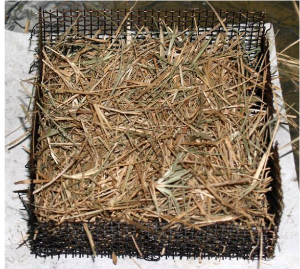
Figure 15. Photograph of cheat grass in cone calorimeter aluminum pan.
