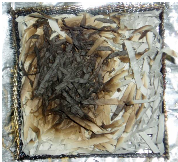
Figure 25. Bottom (left) and top (right) views of a shredded newsprint fuel bed are shown after the fuel was removed from the heated plate held at 333 °C with a low wind applied. Glowing combustion was not observed.
