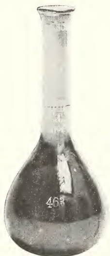
FIG. 7.— Flask for sugar testing
