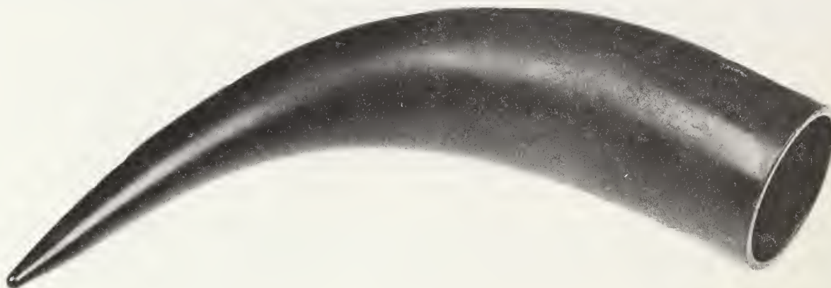
Figure 12.3 A blackbody light trap of glass. The inner surface is coated with a high-gloss black paint having an absorptance of at least ninety-five percent ( \alpha \geq 0.95 ).
