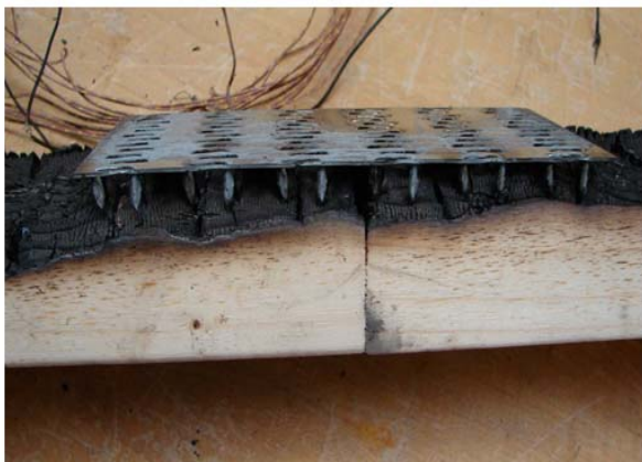
Figure 15 - Post burn - normal specimen
