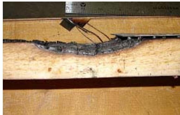
Figure 16 – Char pattern on the left side of the plate.
