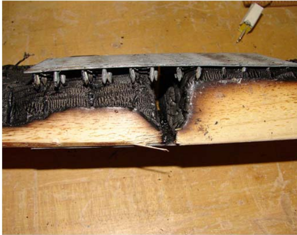
Figure 13 - Post burn - 1/8 in. joint gap specimen
