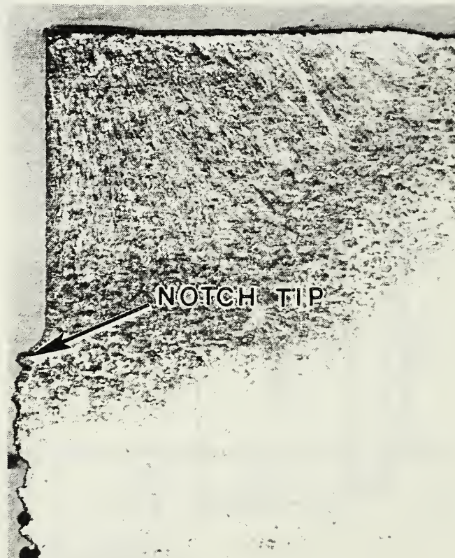
Figure 7.12a - Embrittlement Zone at Notch Tip in Single-Edge Notch Bend Test
