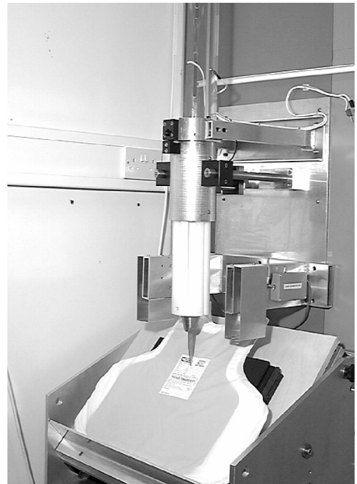
Stab test apparatus used to support development of NIJ body armor standard for stab resistance.
