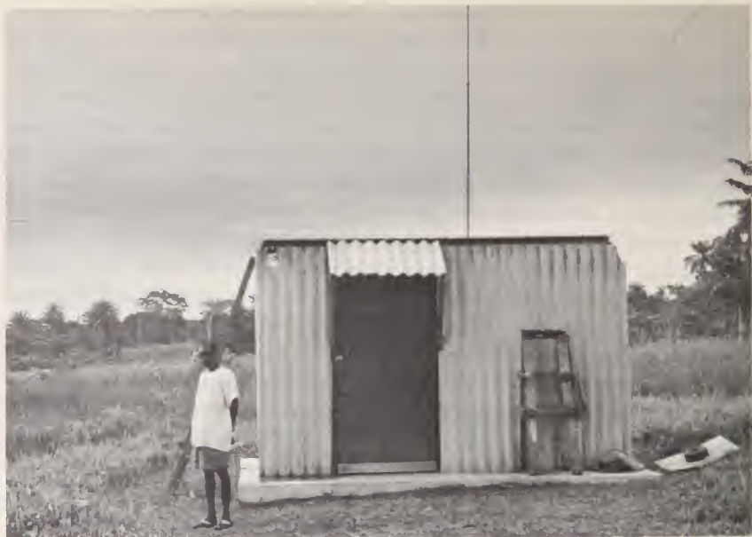
This radio-noise recording station at Ibadan, Nigeria, is one of a worldwide network of noise recording stations. Radio noise data and prediction services assist the telecommunications engineer in the design of facilities that promote the best utilization of the electromagnetic spectrum. (See page 208)
