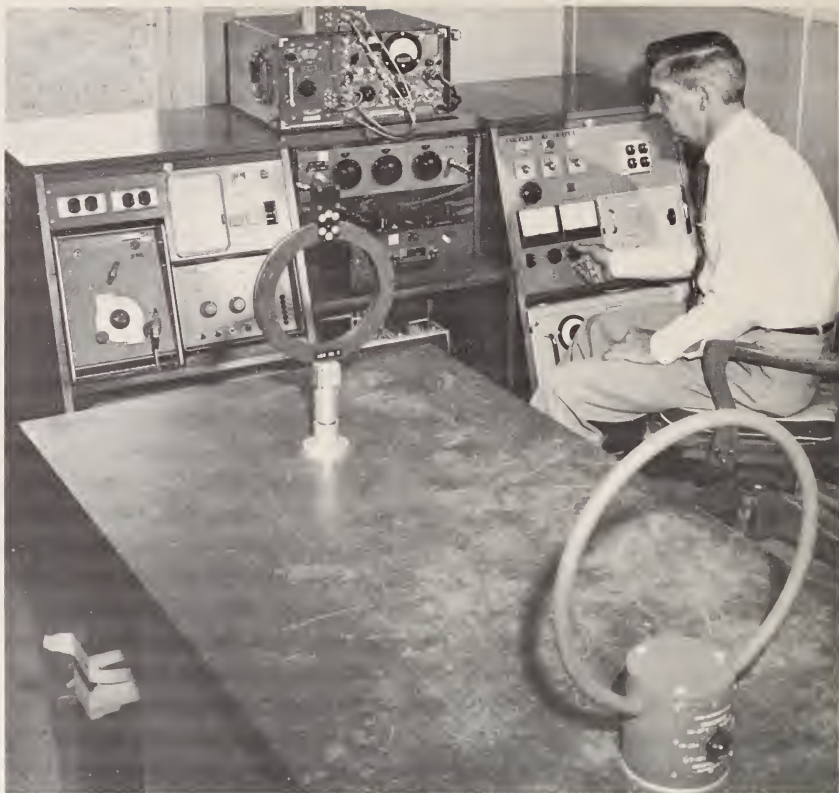
This new calibration console for loop and dipole antennas at 30Hz to 1GHz provides a significant improvement in NBS calibration services.
