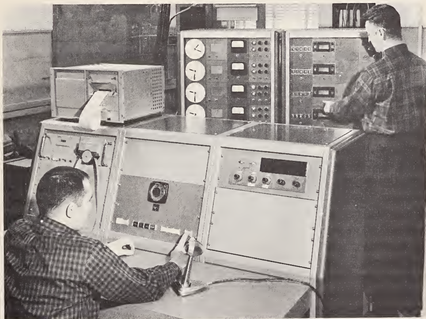
The Vigilometer is used in testing a subject's responses to various visual and auditory stimuli. It was developed for the Army Personnel Research Office to measure attentiveness and fatigue thresholds. (See page 189)
