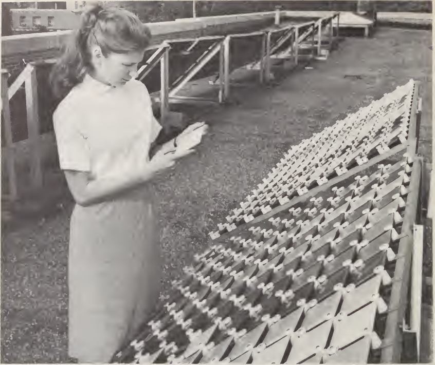
Exposing porcelain enamels on aluminum to determine their durability is part of a current NBS program to develop standard test procedures for such porcelain properties as weather resistance, alkali resistance, and ease of cleaning. (See page 181)
