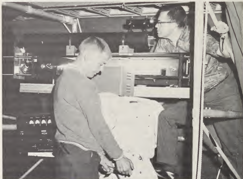
Directing a laser beam from Table Mountain (Boulder) toward Pikes Peak to determine beam fluctuations at long distances. The results of this program should indicate the limitations imposed by the atmosphere on the use of lasers for telecommunications. (See page 216)
