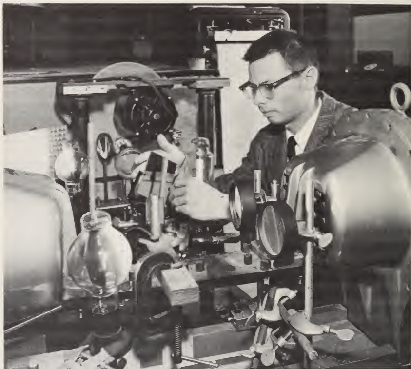
High-resolution infrared spectrometer used to obtain accurate interatomic distances and bonding angles, as well as the physical constants which describe the nature of molecular vibrations. (See page 81)
