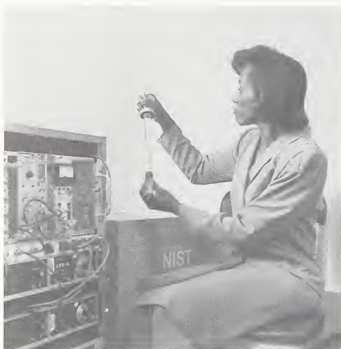
Jacqueline Calhoun places a gamma-ray emitting radionuclide sample into the NIST "4 \pi " \alpha ionization chamber.
