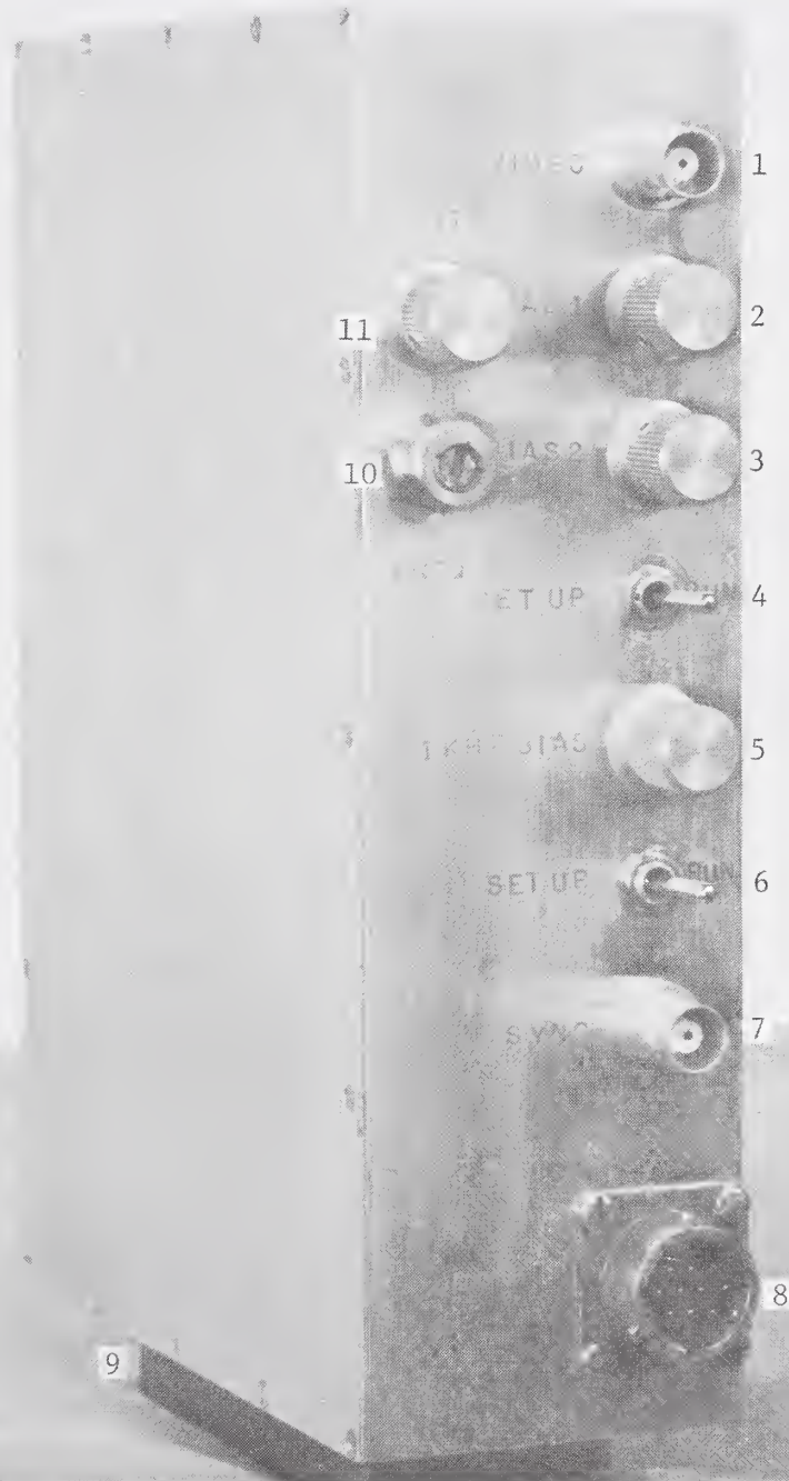
Figure 3.5. Front view of SQUID control unit with index numbers.
