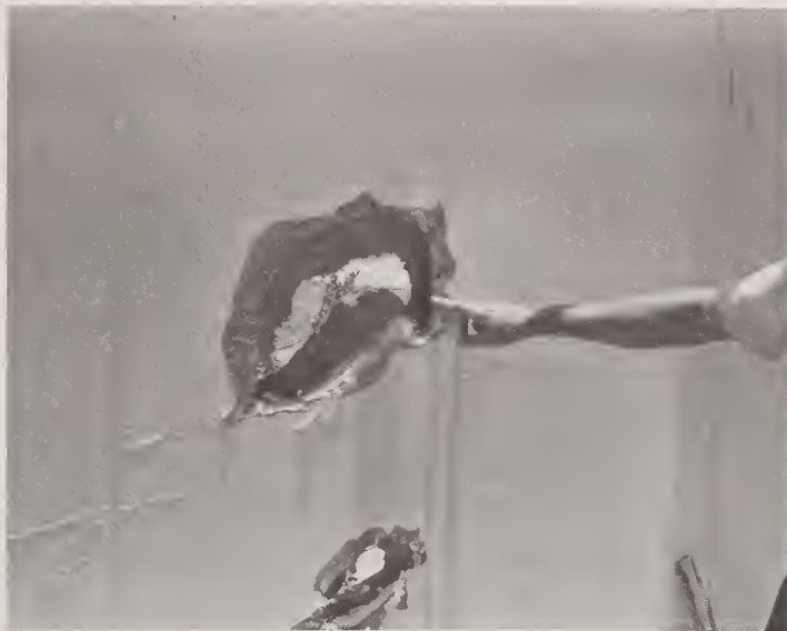
Fig. 33. Missile damage to asbestos cement-polyurethane sandwich panel
