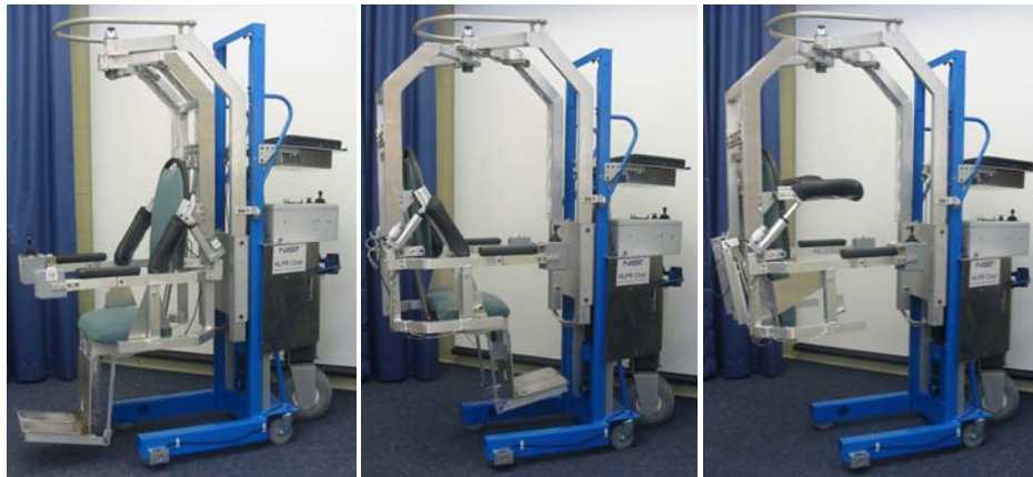
Photographs 4, 5, and 6 (lt. to rt.) of the HLPR Chair prototype in the same configurations as in the graphic above placing a patient on a toilet.
