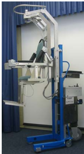
Photograph 7 of the HLPR Chair prototype shown in the patient lift position.
