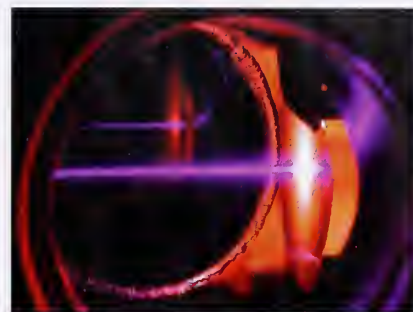
Figure 10. A purple laser beam slows erbium atoms (the purple beam traveling right to left) emerging from an oven at 1300 °C, in preparation for trapping and cooling.
