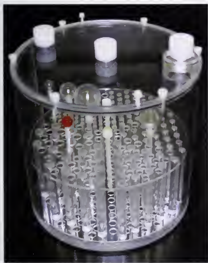
Figure 9. Typical phantom used in clinical quality assurance testing. The red sphere inside the phantom is a NIST prototype demonstrating how calibrated radioactive inserts can be prepared.
