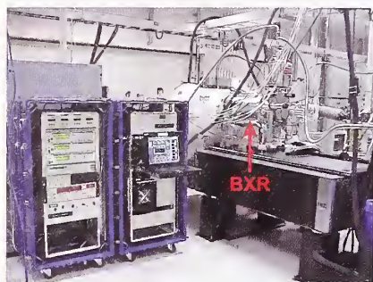
Figure 3. A blackbody standard being calibrated by the NIST BXR in the Exo-atmospheric Kill Vehicle (EKV) missile sensor cryogenic test chamber.
