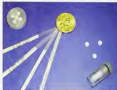
Figure 5. Alanine dosimeters used in radiation processing allow for accurate transfer dosimetry.
