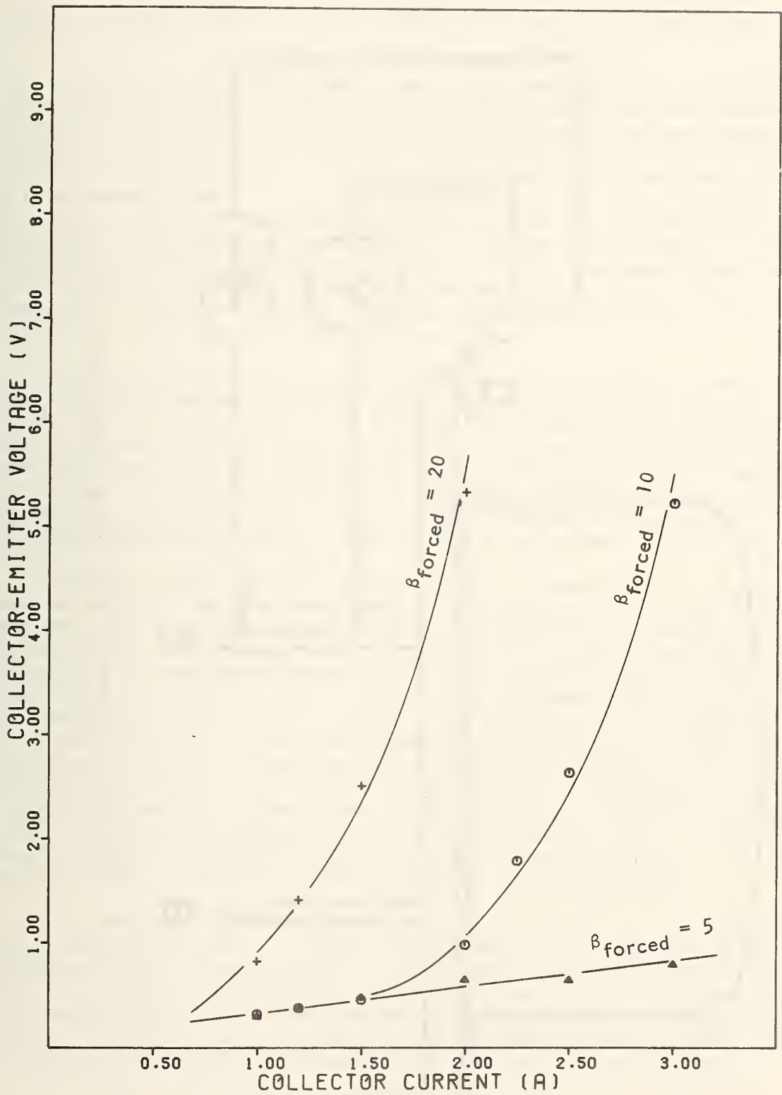
Figure 9c. Collector-emitter voltage as a function of collector current for different values of forced \beta for a 2N5840 transistor.
