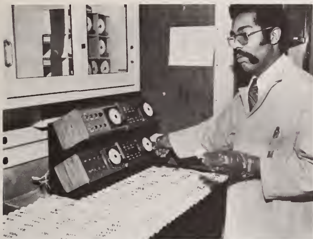
NUCLEAR IRRADIATION FACILITIES. Samples are loaded into pneumatic tubes for transport into the reactor.
