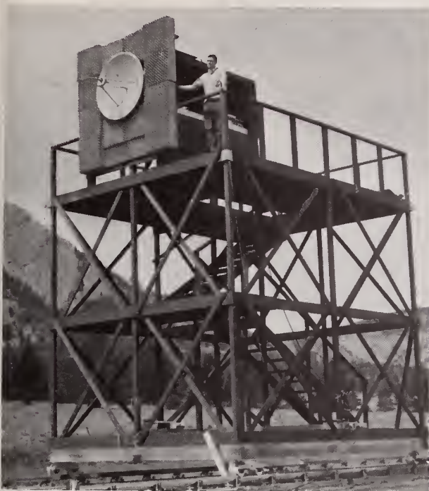
ANTENNA FIELD STRENGTH FACILITIES. Movable towers used for evaluating horn and dish antennas.
