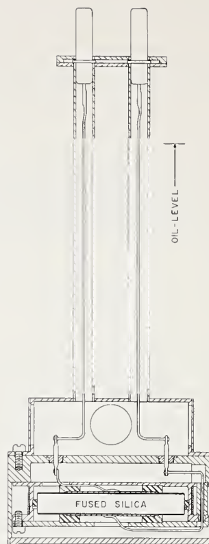
FIGURE 1. Cross section of the capacitance standard.
