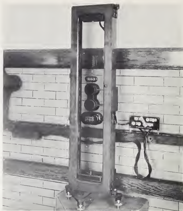
Fig. 1—NBS electrodynamic ac-dc transfer instrument (external multiplier and scale not shown).
