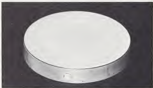
FIGURE 5. Completed fused silica element with an adjustment of minus 50 ppm.
