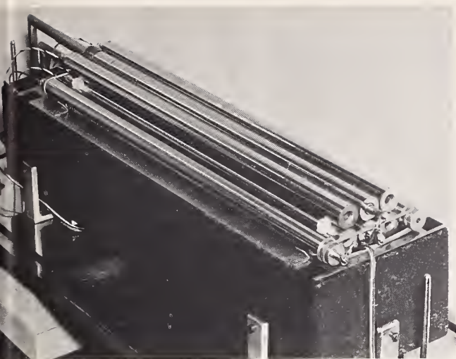
Figure 2. Calculable Cross Capacitor assembled from gage rods.
