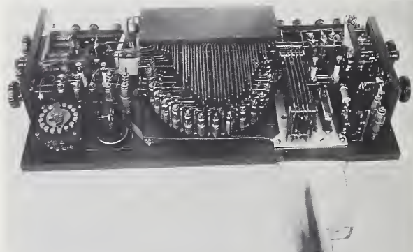
FIGURE 4. Photograph of a Brooks comparator (top view).
