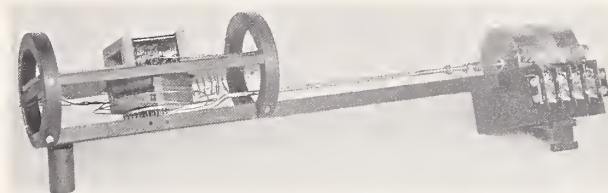
FIGURE 8. Test coil assembly for MH permeameter.
