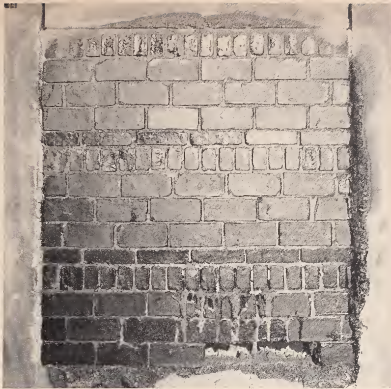
FIGURE 40. Backing side of 12-in. rolok-bak wall 68 after 12-hr 20-min fire test.
