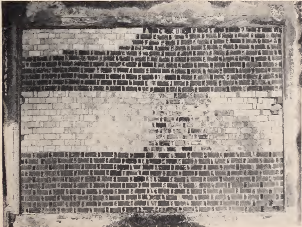
FIGURE 43. Exposed side of 8-in. all-rolok unrestrained wall 77 after fire and hose-stream test.
