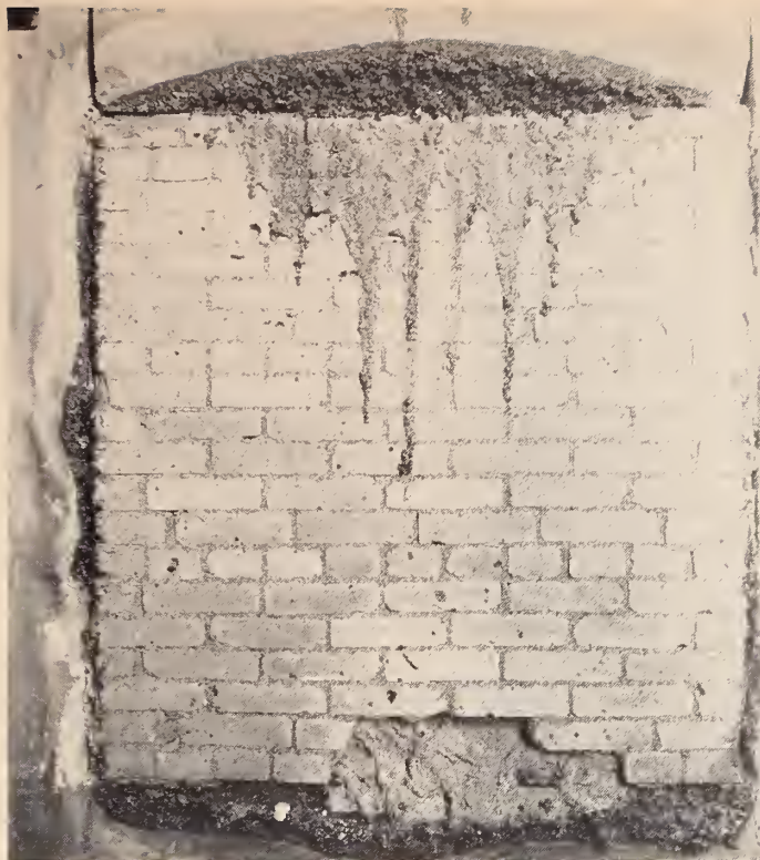
FIGURE 29. Fire-exposed side of 12-in. concrete-brick wall 47 after 16-hr 4-min fire test.
