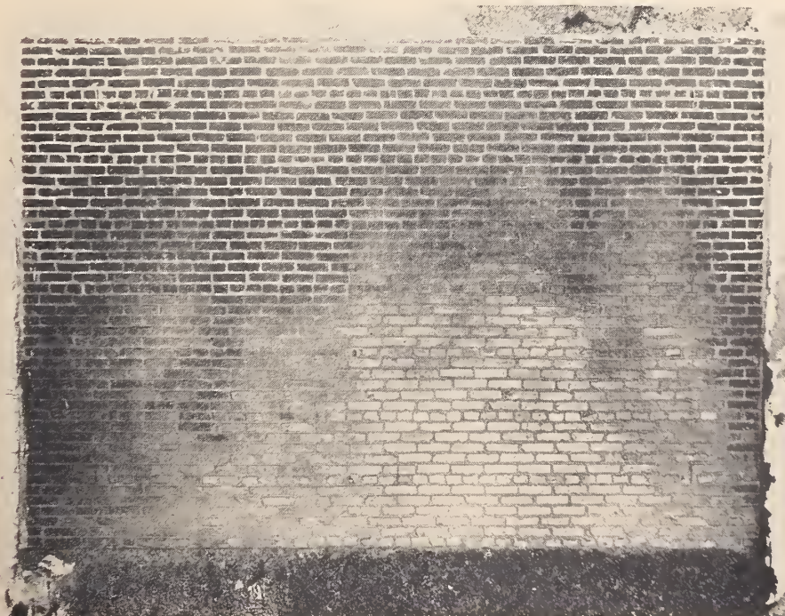
FIGURE 15. Fire-exposed side of wall 11 of clay bricks from source CLM after 6-hr fire test
