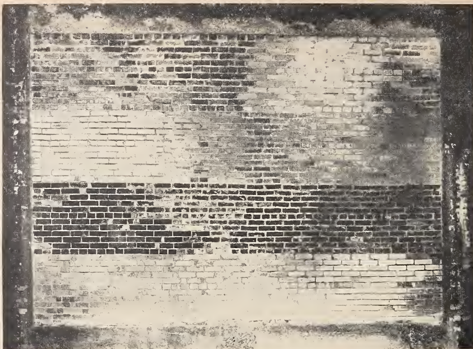
FIGURE 44. Exposed side of 8-in. solid restrained wall 75 after fire and hose-stream test.
