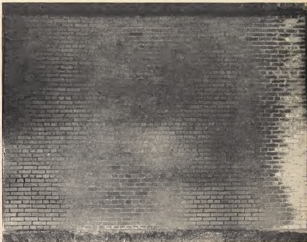
FIGURE 23. Fire-exposed side of 8-in. sand-lime brick wall 30 after 6-hr fire test.
