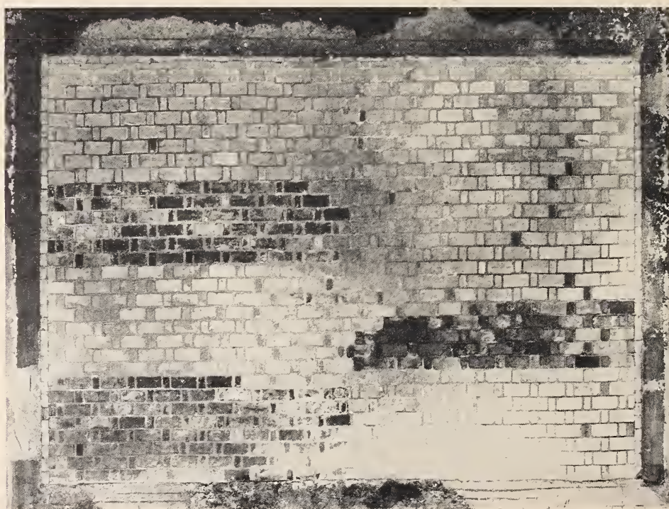
FIGURE 45. Exposed side of 8-in. all-rollok restrained wall 76 after fire and hose-stream test.
