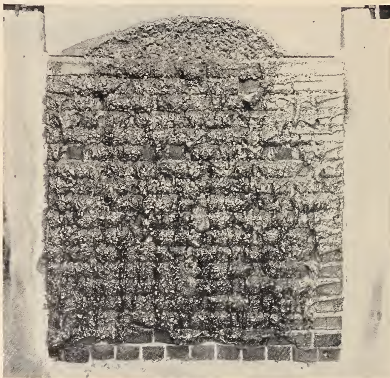
FIGURE 28. Fire-exposed side of 12-in. shale-brick wall 45 after 12-hr 50-min fire test.
