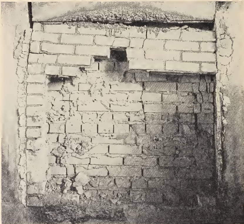
FIGURE 32. Fire-exposed side of 12-in. sand-lime brick wall 52 after failure under load at 9 hr 57 min in fire-endurance test.
