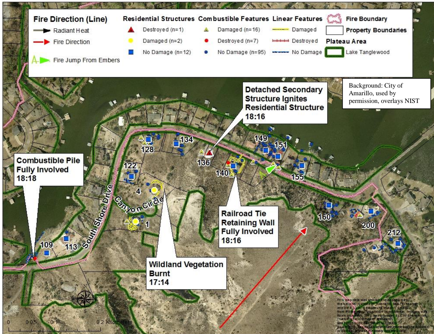
Figure 62 Fire direction and fire timeline in South Lake Tanglewood Community.
