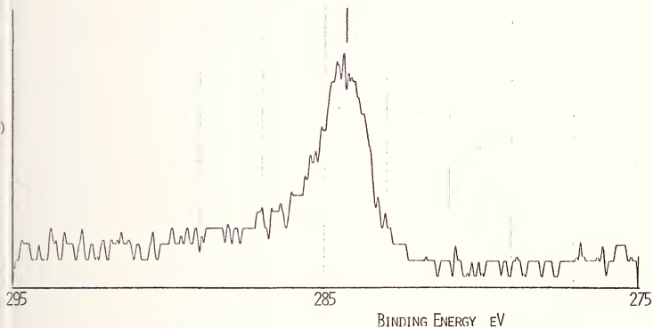
Figure 10. X-ray photoelectron spectrum of the unground carbon 1s peak.
