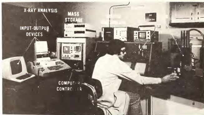
Figure 1. Scanning electron microscope equipped for automatic image analysis as installed in the USS Research Laboratory.
