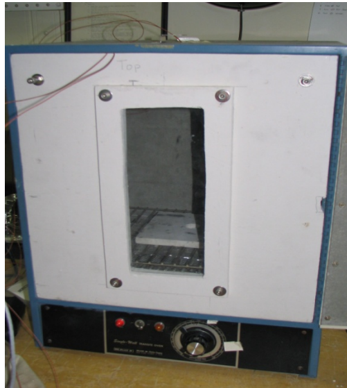
Figure 10. Static oven sealed with a temporary calcium silicate board wall/door.
