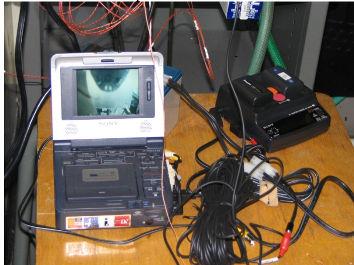
Figure 5. The mini-DV digital video recording unit.
