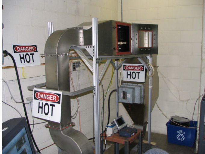
Figure 12. The Fire Equipment Evaluator (FEE) flow loop.
