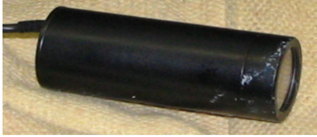
Figure 6. The Sony bullet camera used to record thermal sensing device indicators.
