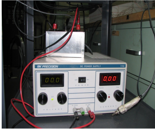
Figure 8. Marker channel power supply and switch.
