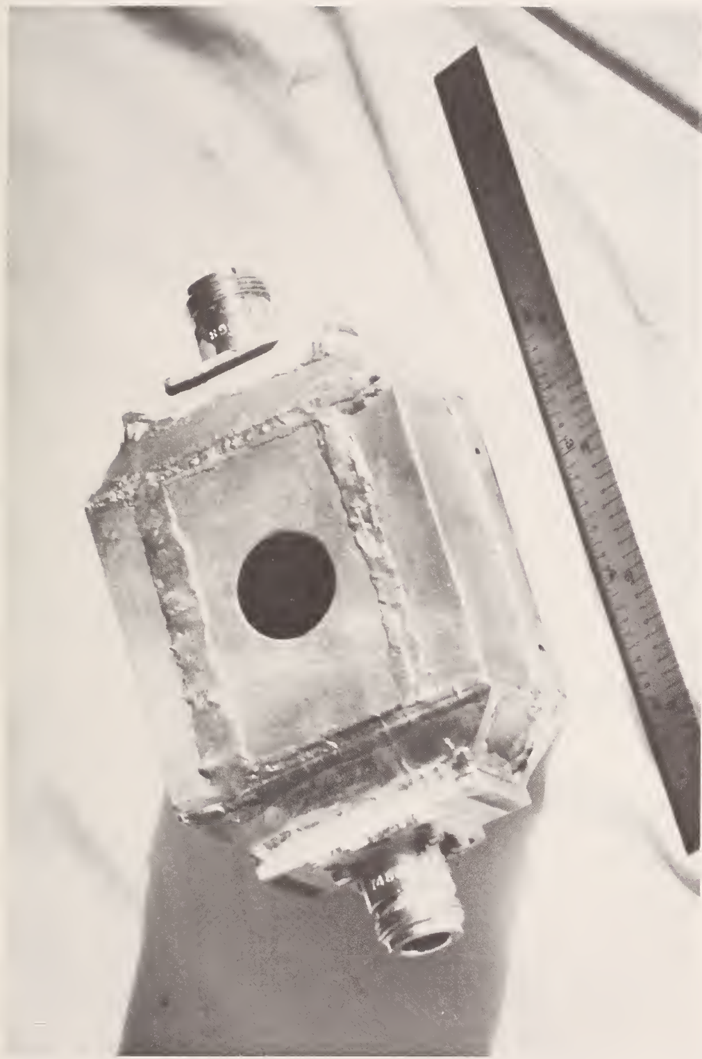
Figure 5.8 Photograph of 3.0 cm x 6.0 cm x 11.4 cm rectangular TEM cell with 1.4 cm diameter aperture.
