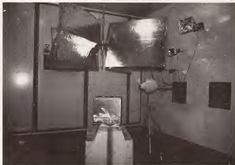
Figure 2.15b Photograph of field tuner/stirrer installed in NSW 3.5 m x 5.2 m x 5.9 m reverberation chamber.
