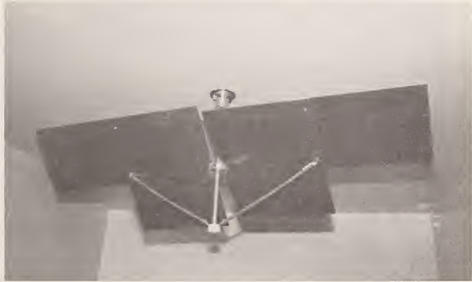
Figure 2.15c. Photograph of field tuner/stirrer installed in NBS 2.7 m x 3.1 m x 4.6 m reverberation chamber.
