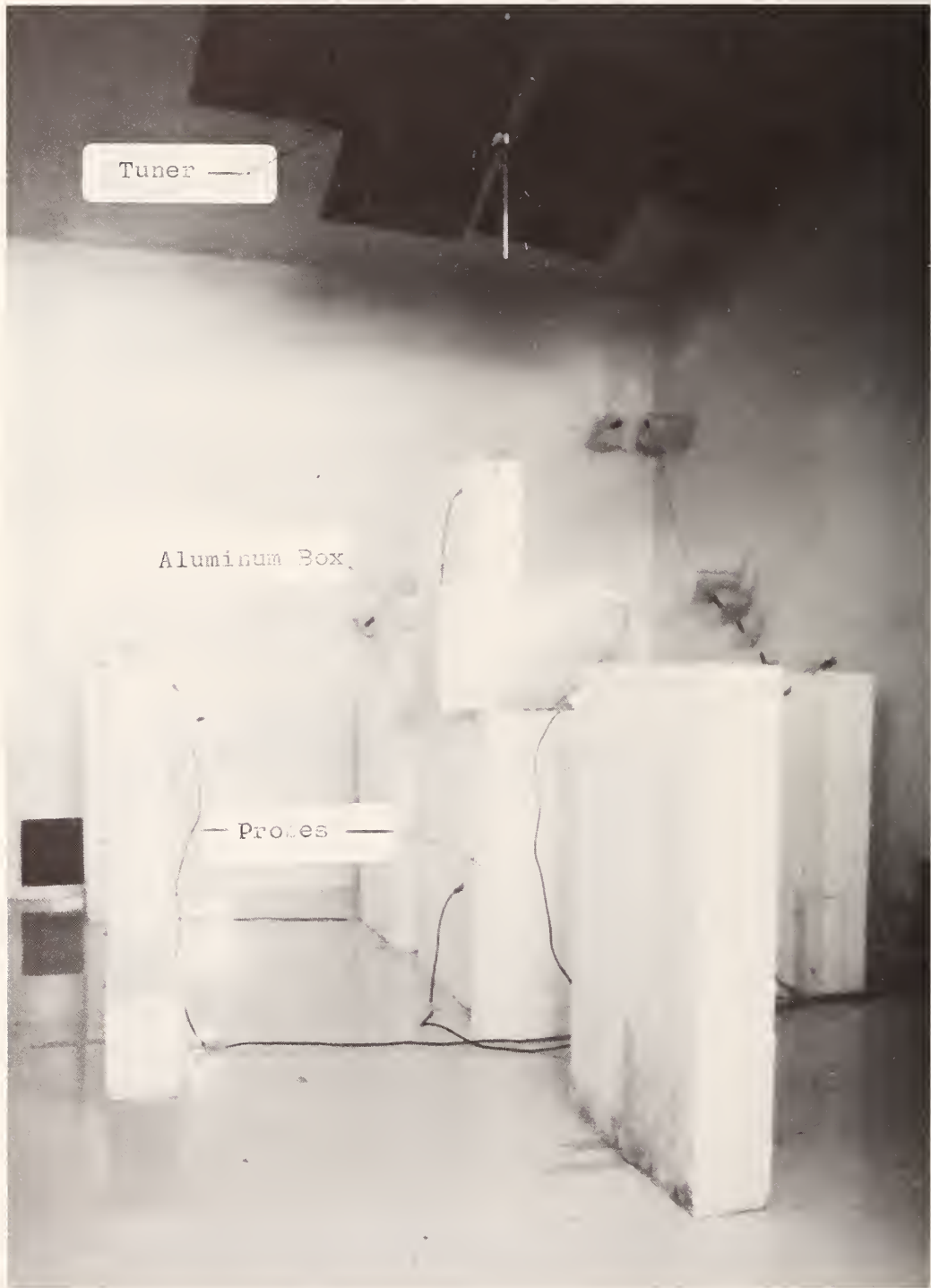
Figure 3.1a Photograph showing 30 cm x 50 cm x 60 cm welded aluminum box inside NBS reverberation chamber.
