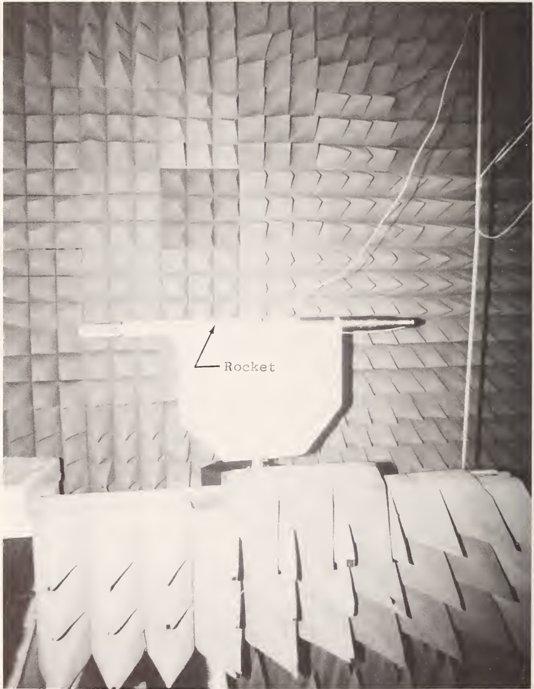
Figure 5.11 Photograph of modified 7.0 cm Folding Fin Aircraft Rocket inside NBS anechoic chamber.
