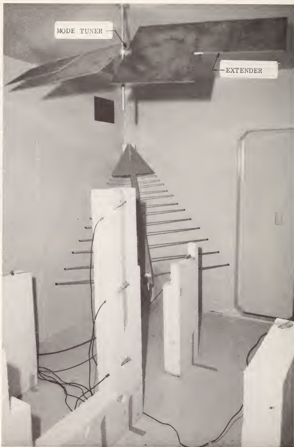
Figure 2.16 Photograph of tuner, log-periodic transmitting antenna and NBS isotropic probes inside NBS reverberation chamber.
